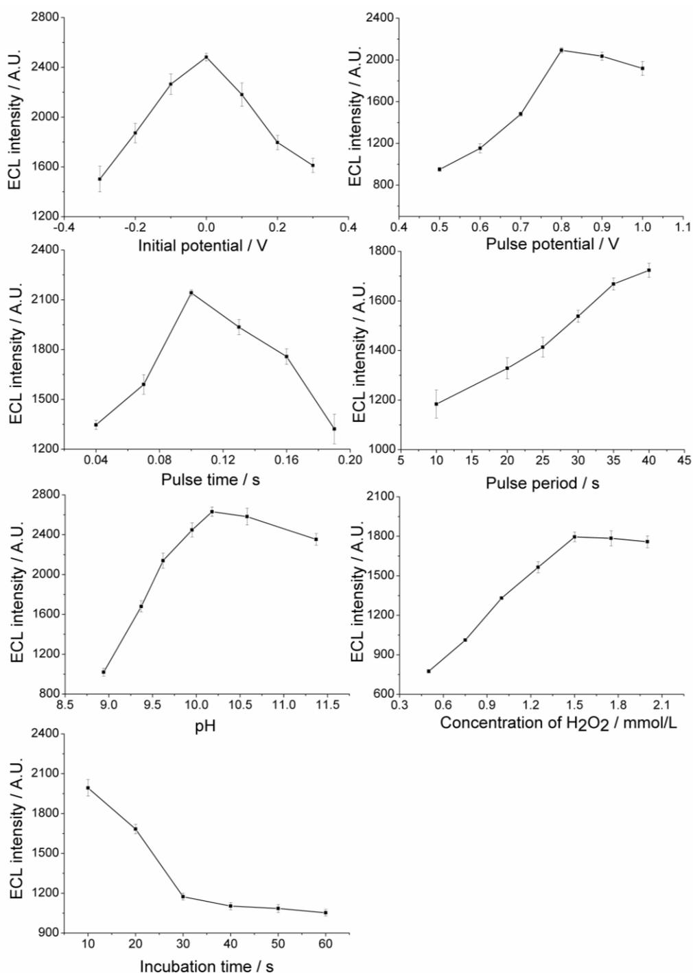
**Fig. S3.** Effects of (a) initial potential, (b) pulse potential, (c) pulse period, (d) pulse time, (e) pH of CBS, (f) H<sub>2</sub>O<sub>2</sub> concentration and (g) incubation time on ECL intensity of the immunosensor. Initial potential, 0 V; pulse potential, 0.8 V; pulse period, 30 s; pulse time, 0.1 s; H<sub>2</sub>O<sub>2</sub>, 1.5 mmol/L; CBS, 0.02 M (pH 10.18), cTnI: 10 ng mL<sup>-1</sup>.
