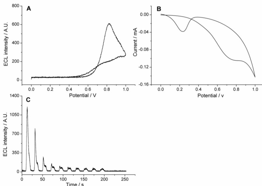
**Fig. S1.** Typical  $I_{\text{ECL}}$ -E curve (A) and cyclic voltammogram (B) of the immunosensor at the scan rate of  $100 \text{ mV s}^{-1}$ . (C) ECL signals of the immunosensor under CV from 0 to 1.0 V, scan rate of  $100 \text{ mV s}^{-1}$ , 10 cycles.  $c_{\text{TnI}}$ :  $10 \text{ ng mL}^{-1}$ .
