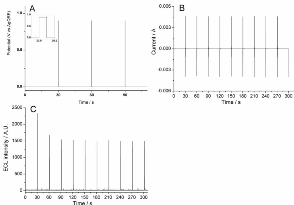
**Fig. S2.** (A) The potential-time curve potential and (B) the current-time curve of the double-step potential applied on the working electrode of the immunosensor. (C) ECL signals of the immunosensor under a double-step potential in 10 pulse periods. Experimental parameters: Initial potential, 0 V; pulse potential, 0.8 V; pulse period, 30 s; pulse time, 0.1 s;  $\text{H}_2\text{O}_2$ , 1.5 mM; CBS, 0.02 M (pH 10.18), cTnI:  $10 \text{ ng mL}^{-1}$ .
