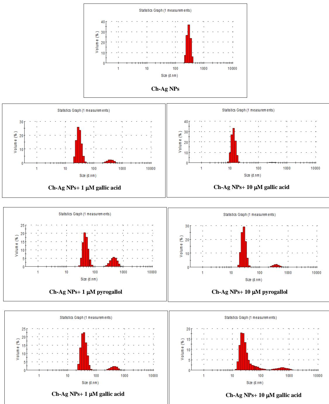
**Fig. S6.** Hydrodynamic diameter distributions of the Ch-Ag NPs in the absence and presence of different concentrations of targets.
