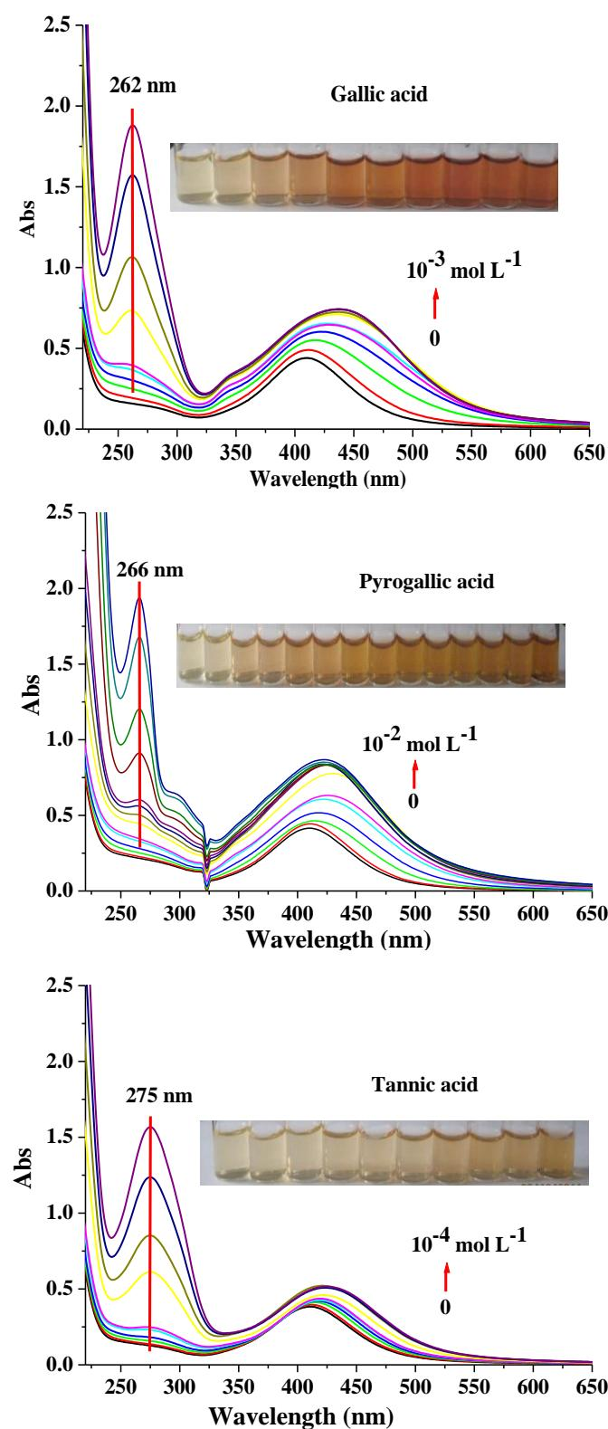
**Fig. S5.** The UV-visible absorption spectra of Ch-Ag NPs colloidal solution in the presence of different concentrations of targets phenols. Inset: photographic images.
