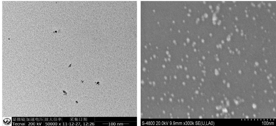
**Fig. S2.** TEM (left) and SEM (right) images of the Ch-Ag NPs.
