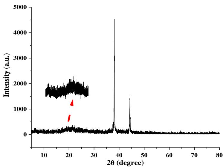
**Fig. S3.** XRD patterns of the Ch-Ag NPs.
