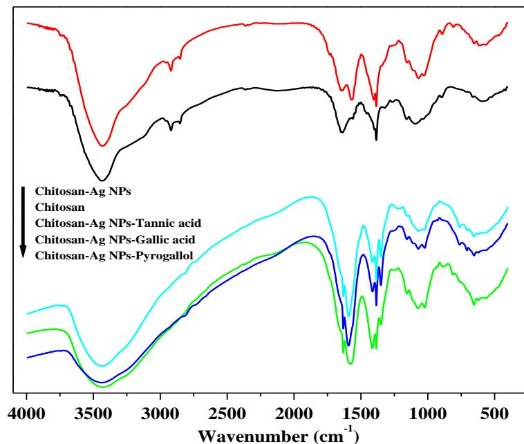
**Fig. S1.** FT-IR spectra of the chitosan, Ch-Ag NPs, Ch-Ag NPs-tannic acid, Ch-Ag NPs-gallic acid, and Ch-Ag NPs-pyrogallol.
