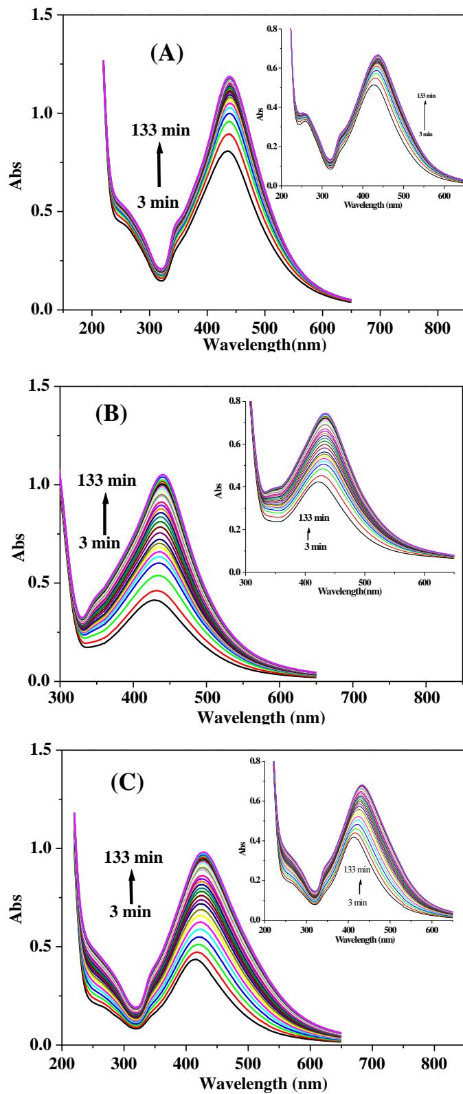
**Fig. S7.** The UV-visible absorption spectra of Ch-Ag NPs colloidal solution with  $\text{AgNO}_3$  in the presence of gallic acid (A), tannic acid (B), and pyrogallol (C). Insets highlight the UV-visible absorption spectra of Ch-Ag NPs colloidal solution in the presence of target without  $\text{AgNO}_3$ . Reaction conditions: 2 mL  $1 \times 10^{-4}$  M Ch-Ag NPs + 0.25 mL  $4 \times 10^{-4}$  M  $\text{AgNO}_3$  or water + 0.25 mL  $2 \times 10^{-4}$  M target compound.
