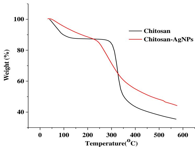
**Fig. S4.** TGA curves of chitosan and Ch-Ag NPs.
