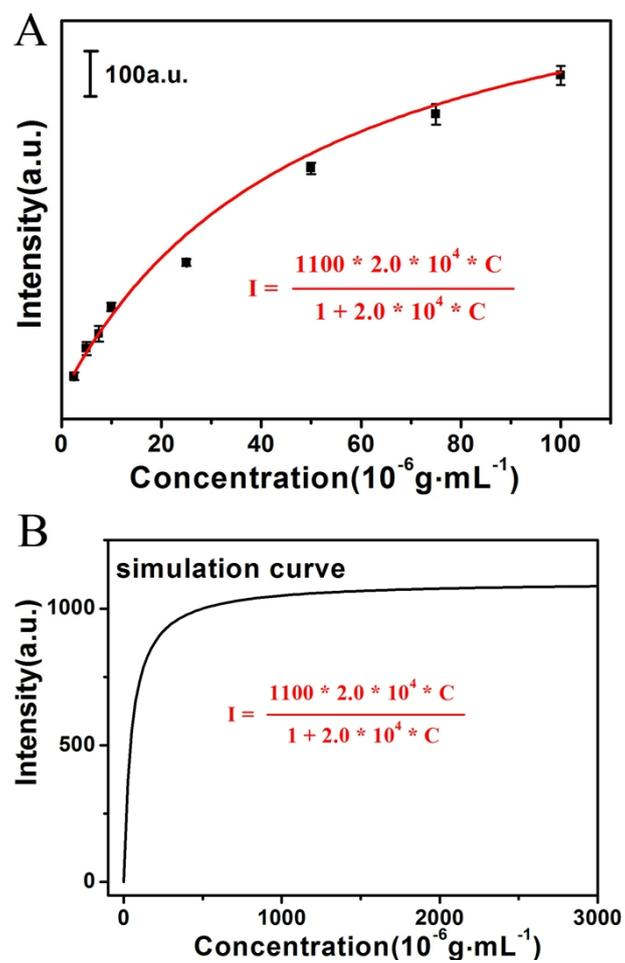
Fig. S10 (A) Plot of the intensity of the 682  $\text{cm}^{-1}$  SERS peak for different melamine concentrations in aqueous solution. (B) Simulation curve of the 682  $\text{cm}^{-1}$  SERS peak for different melamine concentrations in aqueous solution.
