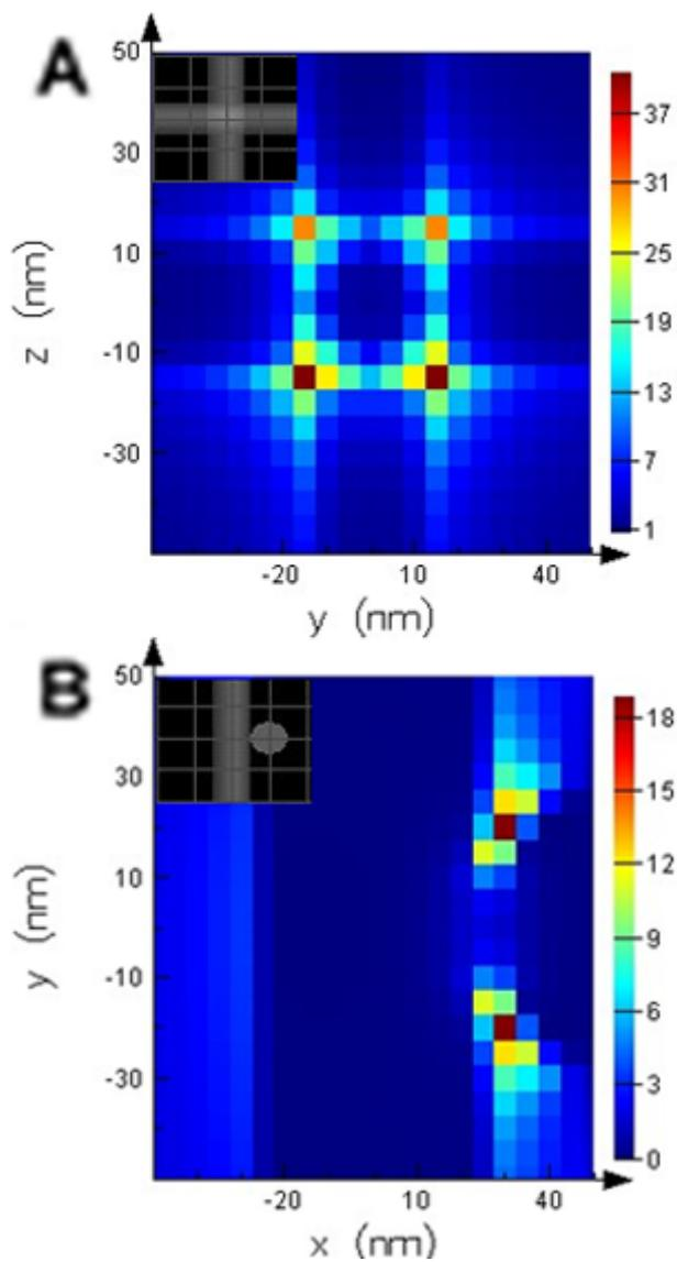
**Fig. S11** Simulated (FDTD) spatial distribution of the electric fields from the y-z (A) and x-y (B) modes of crossed silver nanowires. Inset show the mode of the silver nanowires crossed.
