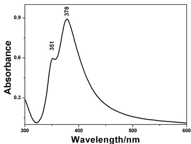
**Fig. S2** UV-Vis absorption spectrum of the silver nanowires.
