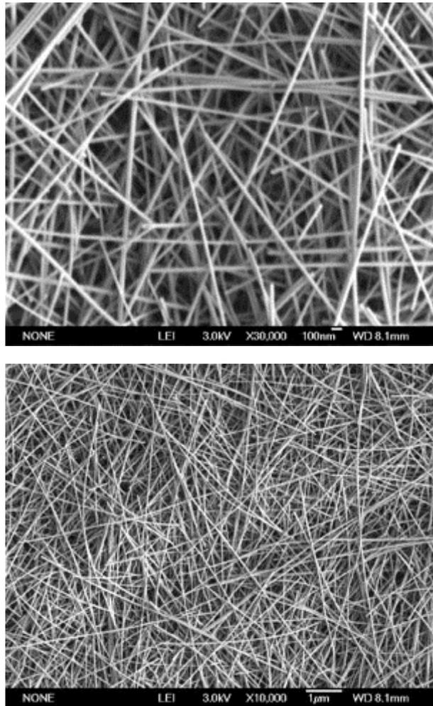
**Fig. S4** SEM image of silver nanowires loaded into the filter membrane.
