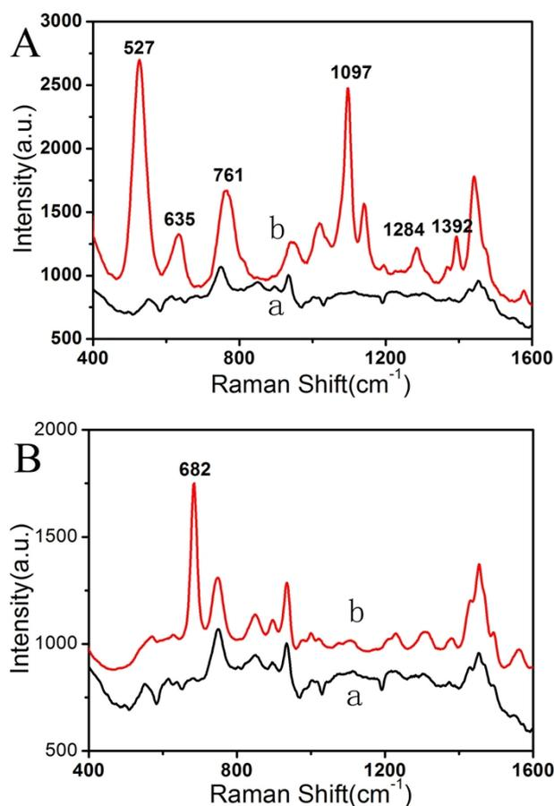
**Fig. S7** SERS spectra of phorate (A) and melamine (B). (SERS spectrum of the blank sample (a))
