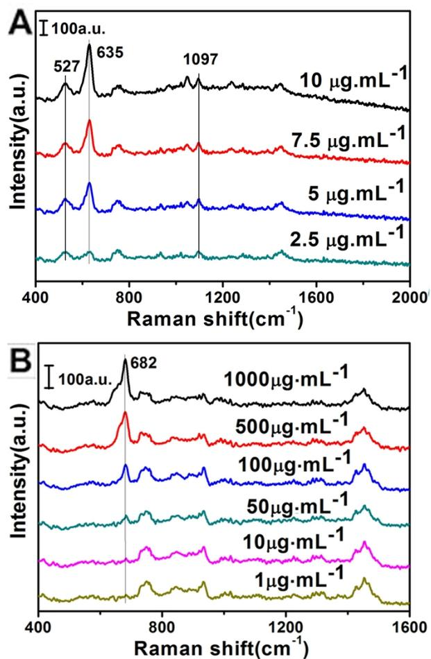
Fig.S12 SERS spectra of (A) phorate and (B) melamine in ground water in the different concentrations by flow-through method.
