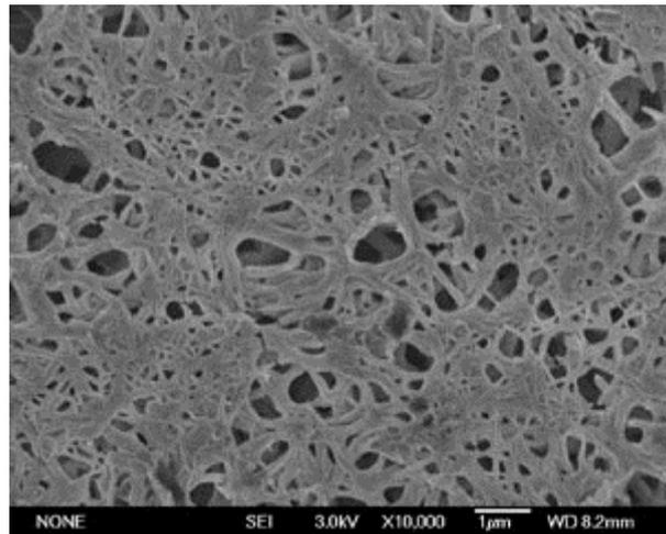
**Fig.S3** SEM image of the membrane without coating silver nanowires.
