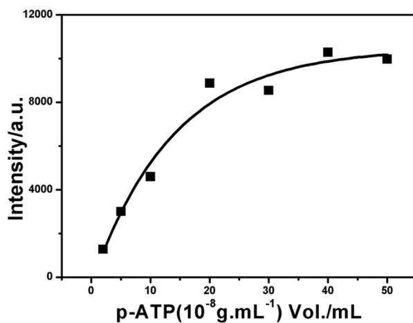
**Fig. S6** Measured intensity of the  $1076 \text{ cm}^{-1}$  PATP SERS peak for increasing volumes of sample loaded into the membrane filter.
