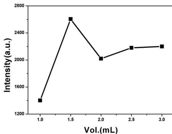
**Fig. S1** Intensity of the 1076  $\text{cm}^{-1}$  PATP SERS peak with different loading volumes of the silver nanowires colloid into the membrane.
