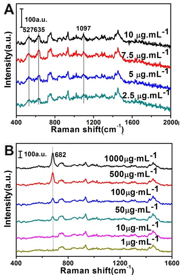
Fig.S13 SERS spectra of (A) phorate and (B) melamine in surface water in the different concentrations by flow-through method.
