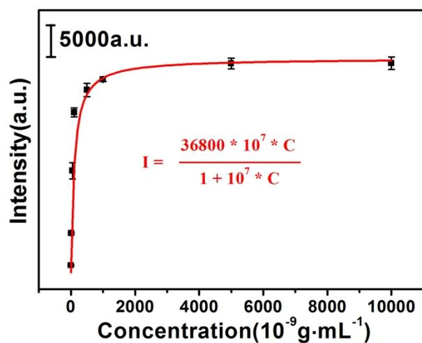
**Fig. S8** Plot of the intensity of the 1076 cm<sup>-1</sup> SERS peak for different PATP concentrations in aqueous solution.
