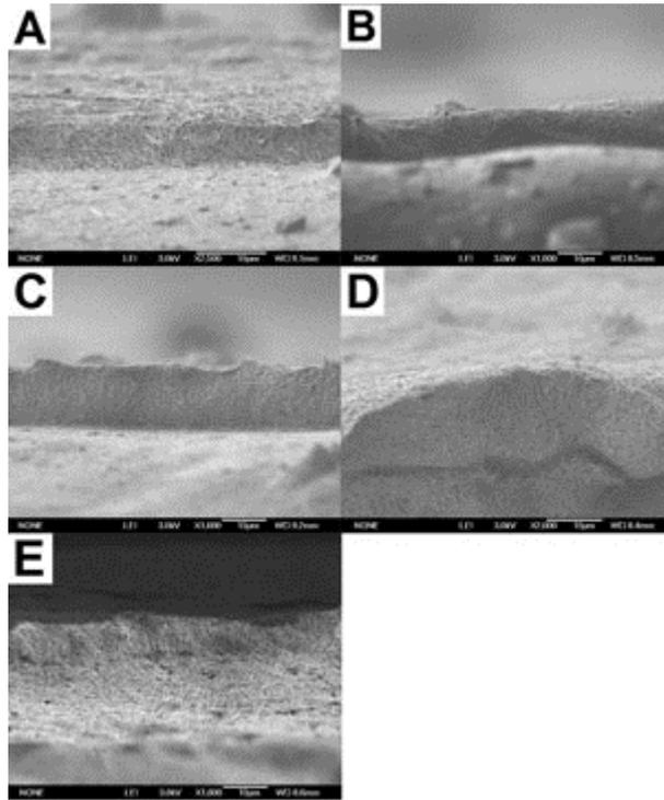
**Fig. S5** Cross-sectional SEM images of the silver nanowires membrane by filtering (A) 1.0 mL; (B) 1.5 mL; (C) 2.0 mL; (D) 2.5 mL; (E) 3.0 mL silver nanowires colloid.
