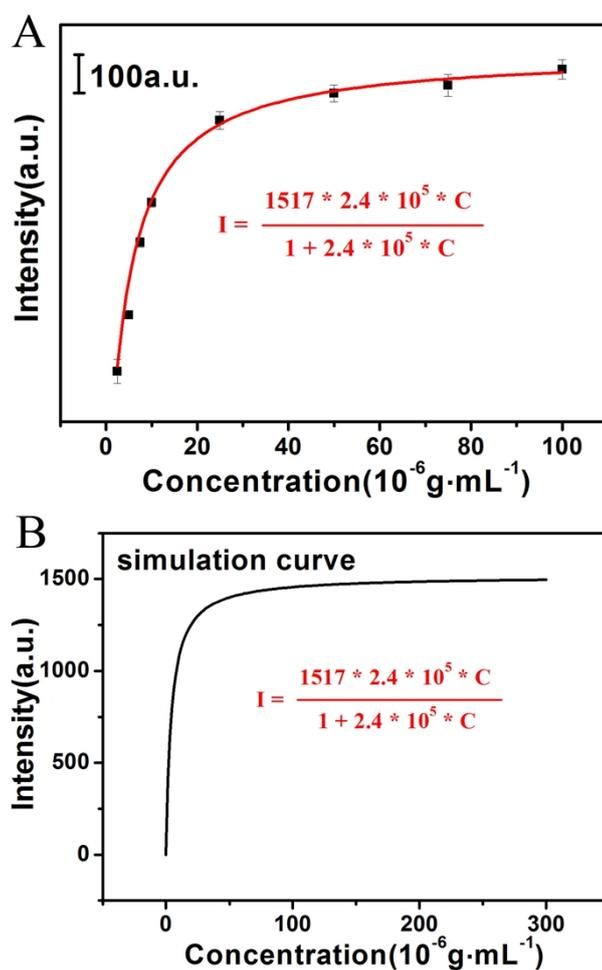
Fig. S9 (A) Plot of the intensity of the 1097 cm<sup>-1</sup> SERS peak for different phorate concentrations in aqueous solution. (B) Simulation curve of the 1097 cm<sup>-1</sup> SERS peak for different phorate concentrations in aqueous solution.
