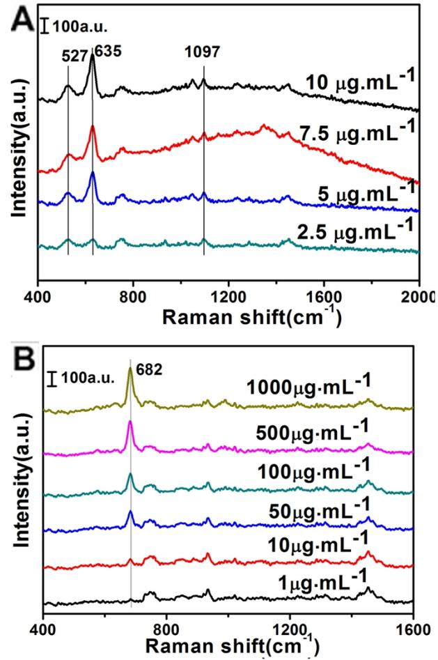
Fig.S14 SERS spectra of (A) phorate and (B) melamine in drinking water in the different concentrations by flow-through method.
