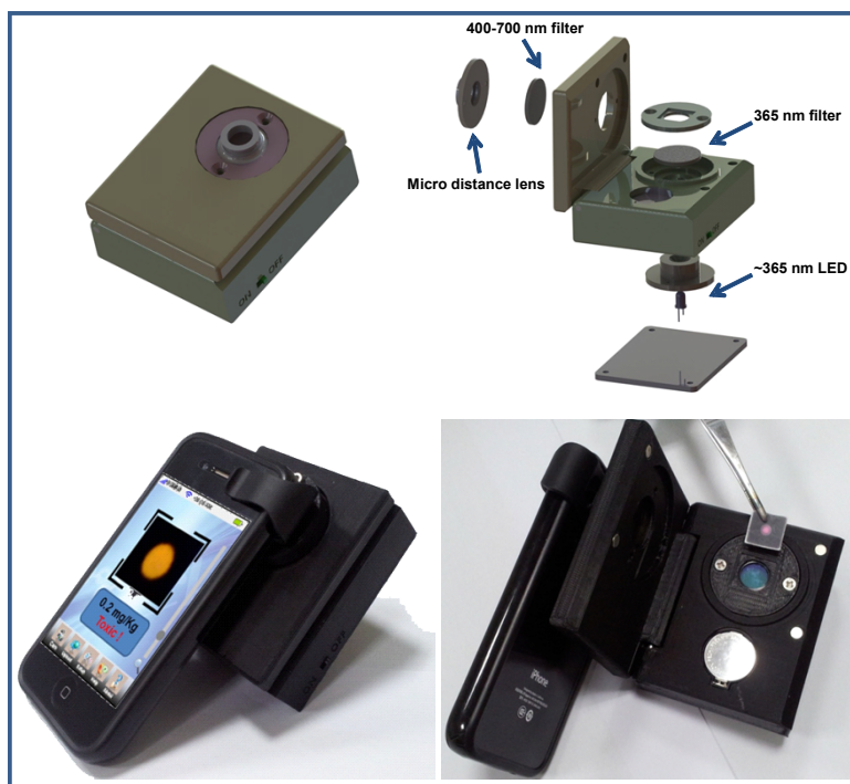
Figure S5. Constructed equipment for BODIPY-based fluorometric paper sensor.
