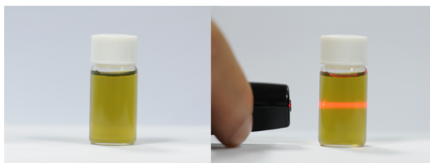
Fig.S1 Left: the suspension of layered MoS 2 nanosheets dispersed in a mixture of water and ethanol. Right: Tyndall effect observed from the MoS 2 suspension.
