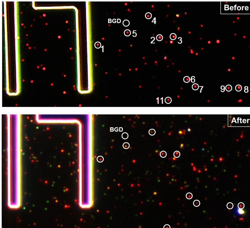
**Figure S2:** Captured microscope images of a chosen area of the grafted glass chip showing the process of AuNT selection before and after each treatment step. The grating was fabricated with a letter and a number in each grid, allowing tracing back of individual AuNTs. Circles around the bright red-dots refer to AuNTs (confirmed by AFM) with a well-defined location, and BGD is the site of measurement of background.
