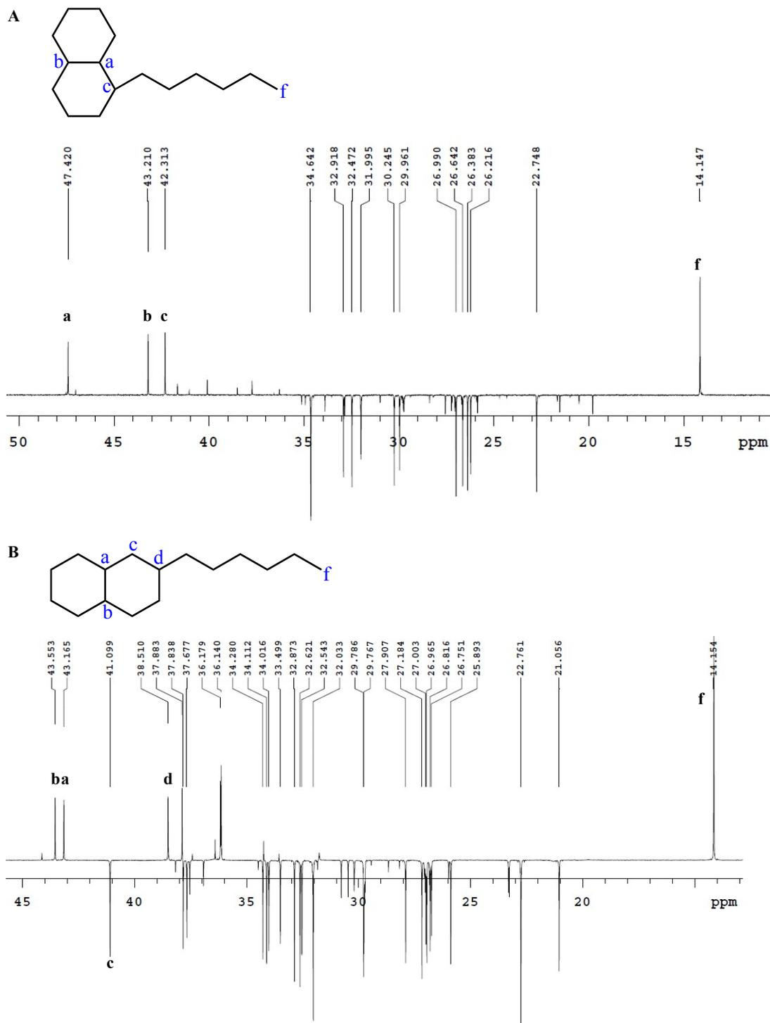
Fig. S1. A)  $^{13}\text{C}$ -NMR DEPT135 spectra of 1-hexyl-decahydronaphthalene; B)  $^{13}\text{C}$ -NMR DEPT135 spectra of 2-hexyl-decahydronaphthalene.
