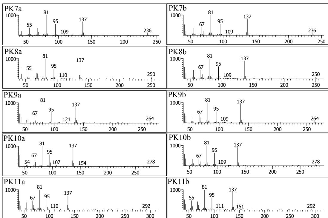
Fig. S3. Mass spectra of PK7a, 7b to PK11a and 11b from the crude oil sample. from the crude oil sample.
