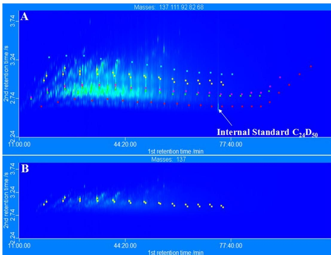
Fig. S2. A) GCxGC-TOFMS EIC ( $m/z$  68+82+92+111+137) showing petrochemical compounds in a rock extracted sample; B) Representative GCxGC-TOFMS EIC ( $m/z$  137) showing the group of pairwise compounds.
