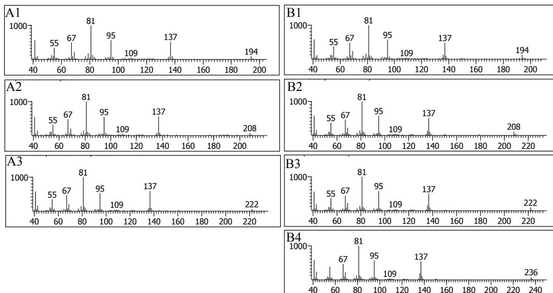
Fig. S4. MS spectra of synthetic 1-alkyl decalins and 2-alkyl decalins. A1) 1-butyl-decahydronaphthalene; A2) 1-pentyl-decahydronaphthalene; A3) 1-hexyl-decahydronaphthalene; B1) 2-butyl-decahydronaphthalene; B2) 2-pentyl-decahydronaphthalene; B3) 2-hexyl-decahydronaphthalene; B4) 2-heptyl-decahydronaphthalene.
