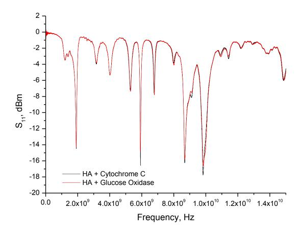
Fig. S3. Reflected signal ( $S_{11}$ ) signal response obtained for a HA modified gold surface with bound glucose oxidase and cytochrome c.
