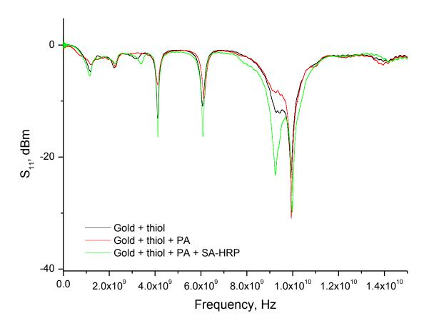
Fig. S1. Reflected signal ( $S_{11}$ ) response obtained for a thiol modified gold surface which was subsequently modified with protein A-biotin and with streptavidin-HRP.
