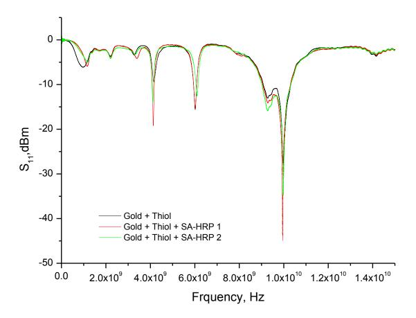
Fig. S2. Reflected signal  $(S_{11})$  response obtained for a thiol modified gold surface which was subsequently modified with protein A-biotin and with streptavidin-HRP.
