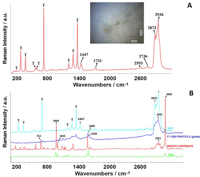
**Figure S-5.** Raman spectrum of brownish spots (see a microscopic detail using the 100x objective lens) on the PTFE sampling support (bands assigned to PTFE are labeled using a T).
