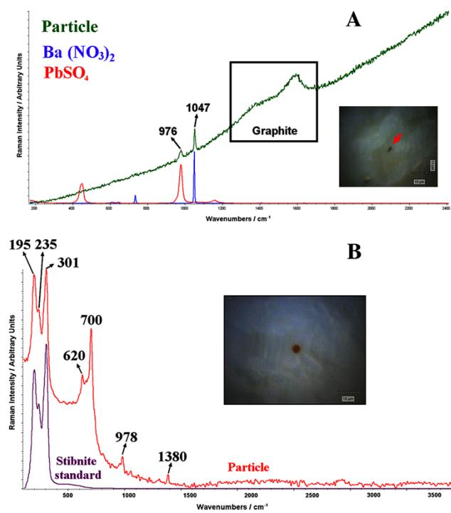
**Figure S-4** A) Raman spectrum of a representative R1 GSR particle (green) (see a microscopic detail of the particle under 100x objective lens) and Raman spectra of nitrobarite (blue) and  $\text{PbSO}_4$  (red) standards. B) Raman spectrum of a representative F2 GSR particle (see a microscopic detail of the particle under 100x objective lens) and Raman spectra of stibnite standards.
