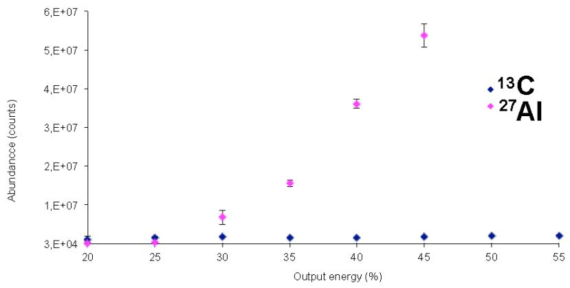
**Figure S-2.** Influence of the laser output energy on the  $^{27}\text{Al}$  and  $^{13}\text{C}$  signals.
