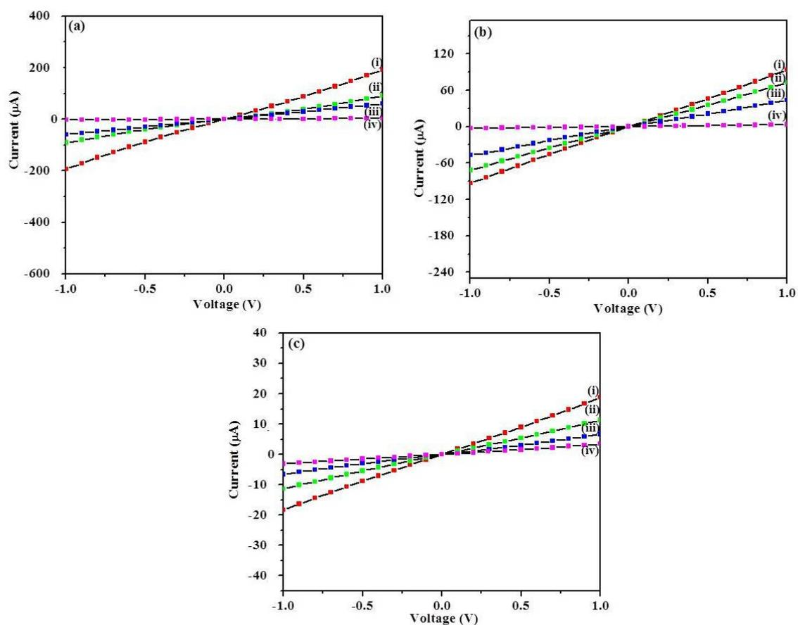
**Supplementary Fig. 2** I-V characteristic graphs of the SWCNT immunosensor with various channel lengths (a) 2  $\mu\text{m}$ , (b) 5  $\mu\text{m}$ , and (c) 10  $\mu\text{m}$  with constant width of 100  $\mu\text{m}$  (i) PDDA-SWCNT, (ii) PDDA-SWCNT-Avidin, (iii) PDDA-SWCNT-Avidin-biotinylated antibody, and (iv) PDDA-SWCNT-Avidin-biotinylated antibody-H1N1 virus.
