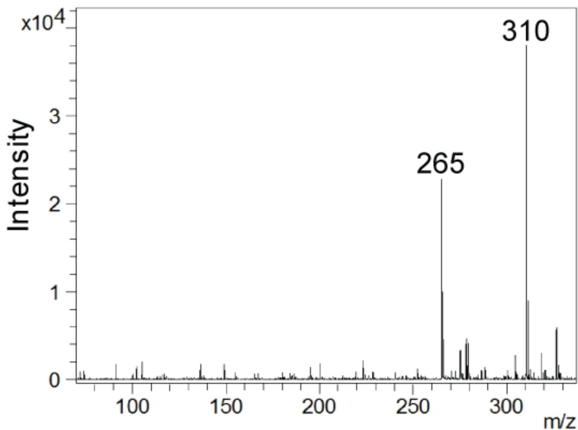
**Figure S-3.** Representative SALDI mass spectra on SiNP arrays etched in a 4.8 M HF/0.1 M H<sub>2</sub>O<sub>2</sub> solution for 1 min (450 nm in length, 450 nm diameter, 100 nm inter-nanopillar spacing, and an aspect ratio of 1.0) for methadone with a MH<sup>+</sup> = 310 m/z. Another peak appearing at 265 m/z was identified as a methadone fragment.
