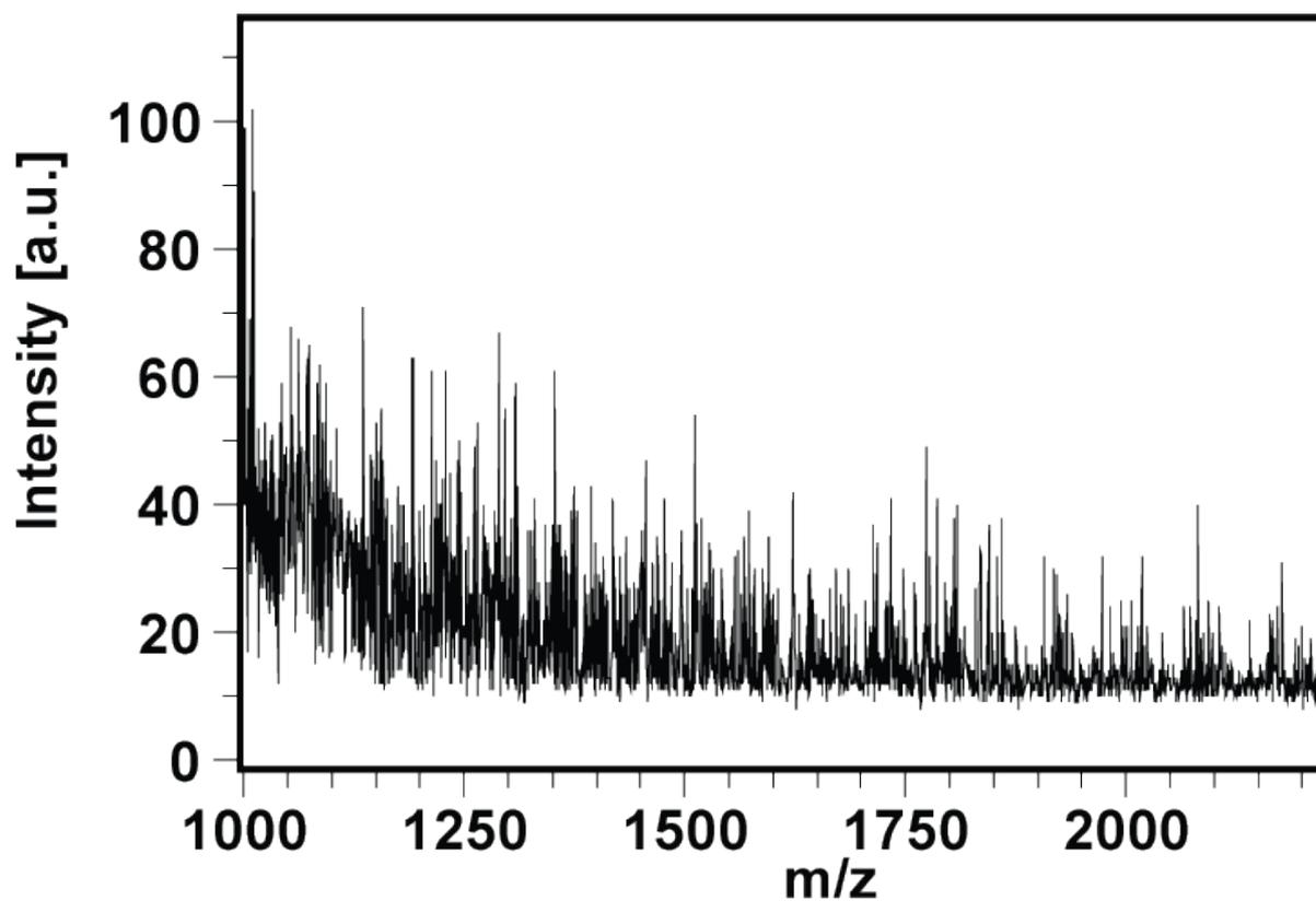
**Figure S-2.** SALDI-MS spectrum collected of a MilliQ water droplet that did not contain any peptides. The substrate used was a SiNP array etched for 1 min using a solution of 4.8 M HF/0.1 M H<sub>2</sub>O<sub>2</sub>.
