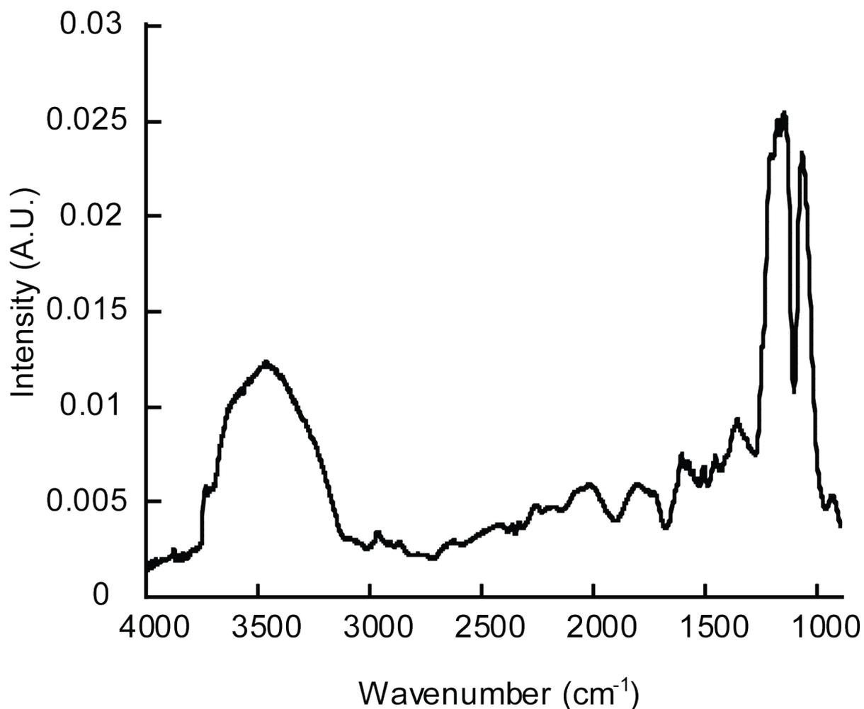
**Figure S1.** FTIR spectrum collected using Diffuse Reflectance Infrared Fourier Transform (DRIFT) on SiNP arrays. The SiNP array was taken after fabrication directly without any further modification and analyzed. In the sample spectrum, Si-O-Si and Si-OH characteristic peaks can be observed at 1050-1200 and 3745 (cm<sup>-1</sup>), respectively. Additionally, a broad peak characteristic of bonded -OH was present between 3100 and 3600 cm<sup>-1</sup>.
