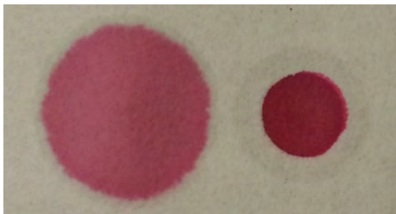
Figure 5S: Difference in spreading efficiency of a 15 \mu L aqueous solution unconstrained (left) and constrained (right) by a silicone barrier.
