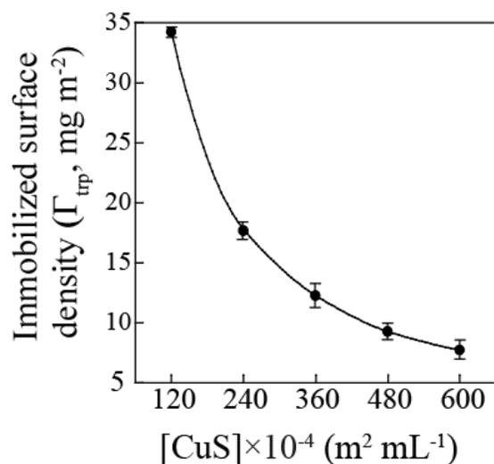
**Fig. S6.** Adsorption capacity of trypsin on CuS nanoparticles as a function of available nanoparticle surface area. Increasing amount of nanoparticle surface area for binding were made available ( $120 \times 10^{-4}$  to  $600 \times 10^{-4} \text{ m}^2 \text{ mL}^{-1}$ ), by adding 0.2 – 1.0  $\text{mg mL}^{-1}$  of CuS nanoparticles to  $0.1 \text{ mg mL}^{-1}$  of trypsin solution.
