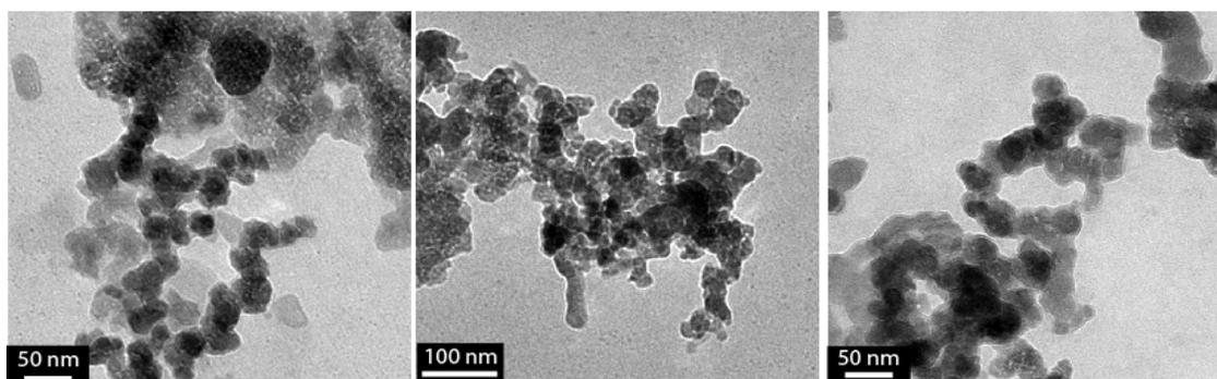
**Fig. S1.** Additional TEM images of CuS nanoparticles (20-50 nm).
