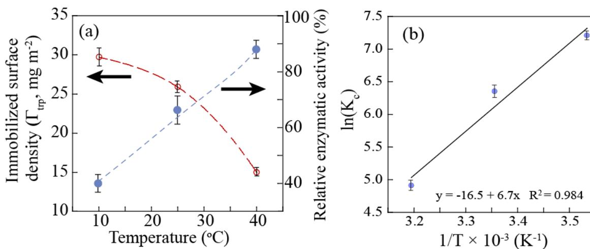
**Fig. S9.** Influence of temperature on trypsin interaction with CuS nanoparticles: (a) trypsin adsorption capacity (red) and enzymatic activity (blue) at different temperature. (b) Van't Hoff plot of trypsin molecules adsorbed on CuS nanoparticles. The Van't Hoff equation is expressed by:
