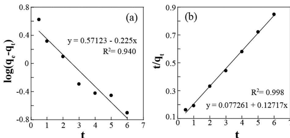
**Fig. S5.** Adsorption kinetics of trypsin on CuS nanoparticles analyzed by (a) first order and (b) second order kinetic model.
