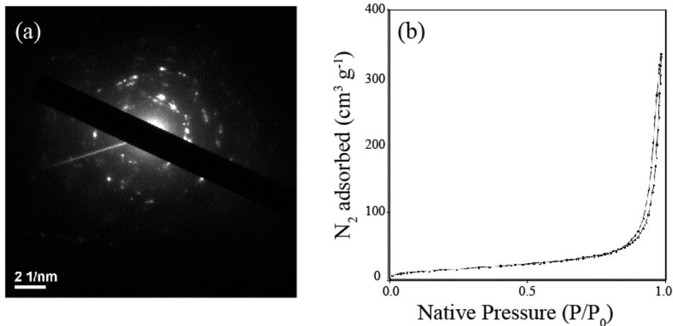
**Fig. S3.** (a) Selective area electron diffraction (SAED) of CuS nanoparticles; and (b) N<sub>2</sub> adsorption/desorption isotherms of CuS nanoparticles measured from BET analysis.
