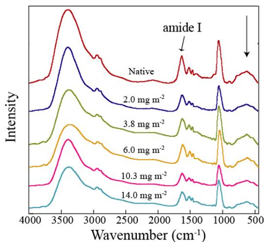
**Fig. S7.** FT-IR spectra of free trypsin and after interaction with CuS nanoparticles in 4000-450  $\text{cm}^{-1}$  of range (Arrow indicates the Amide I region which has been further used for Gaussian distribution analysis). Top graph represents the FT-IR spectra of native trypsin, and the followings are the FT-IR spectra of immobilized trypsin at different surface coverage ( $\text{mg m}^{-2}$ ).
