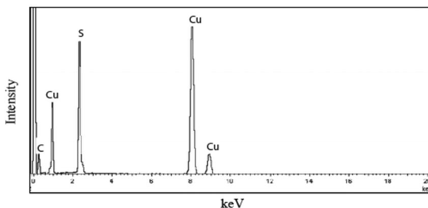
**Fig. S2.** Energy-dispersive X-ray (EDX) spectrum of synthesized CuS nanoparticles, showing the presence of Cu and S.
