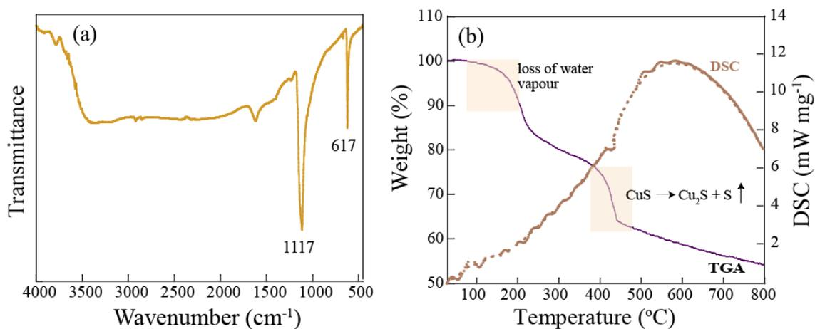
**Fig. S4.** (a) FT-IR spectra of CuS nanoparticle is taken in the range of 4000-450 cm<sup>-1</sup>, with a scan number of 20 (scan resolution 4cm<sup>-1</sup>); and (b) Thermogravimetric (TGA-DSC) analysis of CuS nanoparticles.
