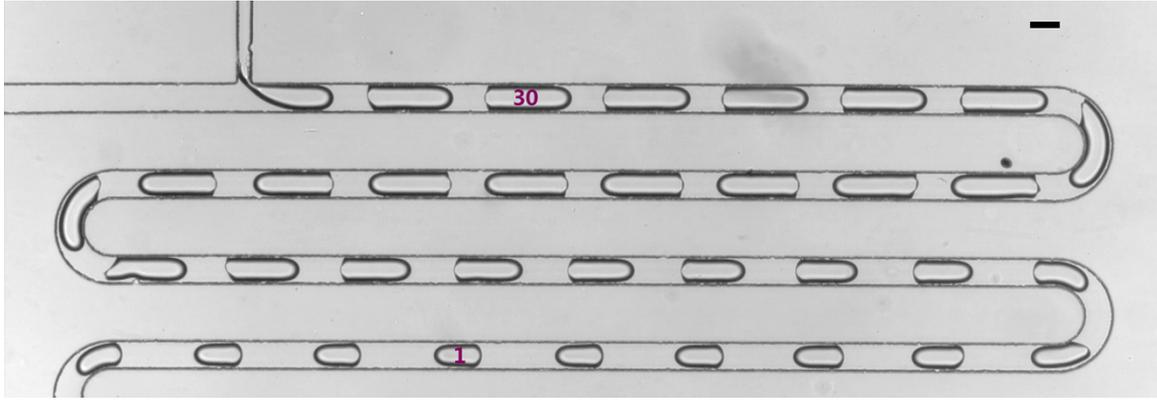
**Figure S6** Droplet size gradient in T-junction. The smallest droplet is marked as (1) and the largest as (30). The scale bar is 100  $\mu\text{m}$ .
