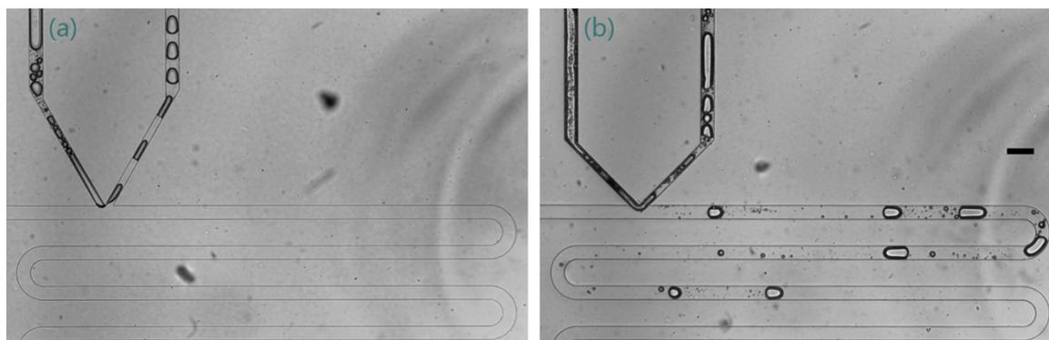
**Figure S4** Comparison of *open-mode* reliability for the 60° and 90° V-junction designs. The 90° chip (b) already fails at flow-rates of 2  $\mu\text{l}/\text{min}$  oil and 1  $\mu\text{l}/\text{min}$  water (0.5 ratio) while 60° chip (a) is competent in the same condition. The scale bar is 200  $\mu\text{m}$ .
