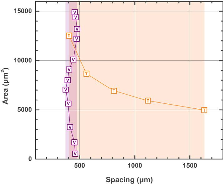
**Figure S8** Plot of droplet spacing versus droplet area for V- and T-junctions.
