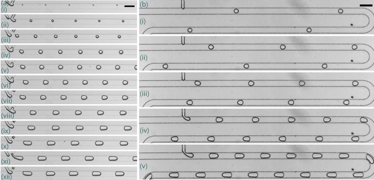
**Figure S7** Comparison of frequency and spacing between droplets produced in (a) V-junction and (b) T-junction. The scale bars are 200  $\mu\text{m}$ .
