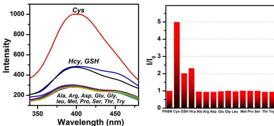
**Figure S7.** Left: Fluorescence excitation spectra of **PHSN** (5 μM) against 40 equivalents of Cys, Hcy, GSH and various other amino acids in HEPES buffer (50% EtOH v/v, pH 7.4) at 37.4 °C. Right: Corresponding histogram demonstrated the selectivity of **PHSN** for Cys over other amino acids.
