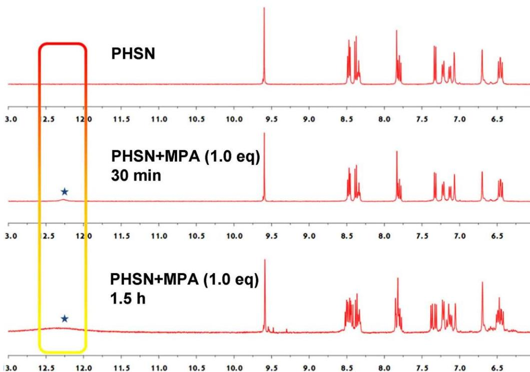
**Figure S5.**  $^1\text{H}$  NMR spectra of PHSN with MPA for 30 min and 1.5 h, the spectra was shown from 13.0 to 6.0 ppm. The small peaks marked by stars showed the appearance of carboxyl proton.
