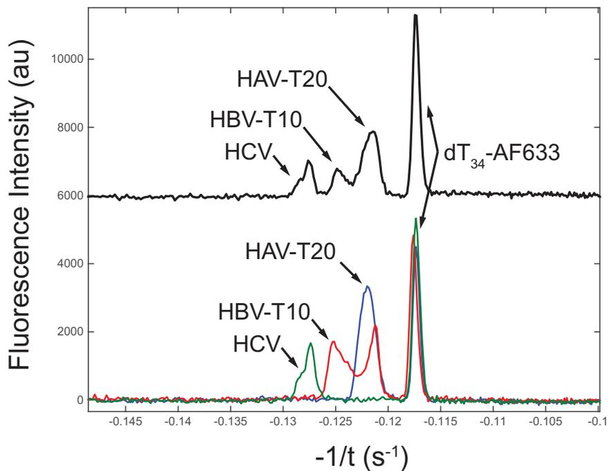
Figure S7: mCE separation of a sample mixture containing probe+target for HAV-T20, HBV-T10, HCV and a poly- $dT_{34}$  reference peak with an Alexafluor633 tag. The HBV-T10 probe+target complex produces two elution peaks indicating that there are two stable conformations that yield similar AgNCs. However, improved separation resolution is necessary to separate the secondary HBV-T10 peak and the HAV-T20 and eliminate a false-positive for HAV target in the presence of HBV target.
