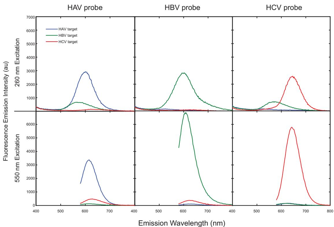
Figure S2: Emission spectra of each probe in the presence of all three different DNA targets. Top row shows emission at 260 nm excitation. Bottom row shows emission at 550 nm excitation. Each probe shows bright fluorescence in the presence of its complementary target and weak to no fluorescence when in the presence of mismatched target. Excitation at 550 nm further minimizes any fluorescent emission from probes with mismatched targets.
