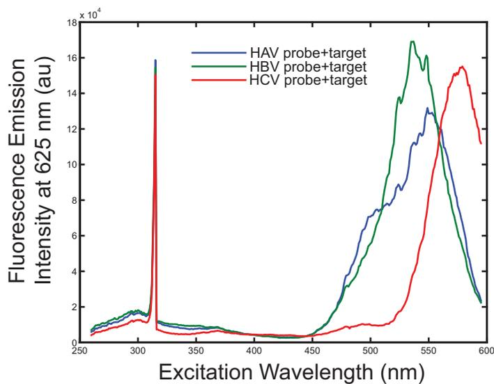
Figure S3: Fluorescence excitation scan of AgNC-DNA probes for HAV, HBV and HCV in the presence of their respective target DNA. The detector is set to an emission wavelength of 625 nm. The large spike near 312 nm is an artifact related to a harmonic of the detector wavelength, 625 nm. These spectra show that excitation at 550 nm produces approximately equal emission for each probe.
