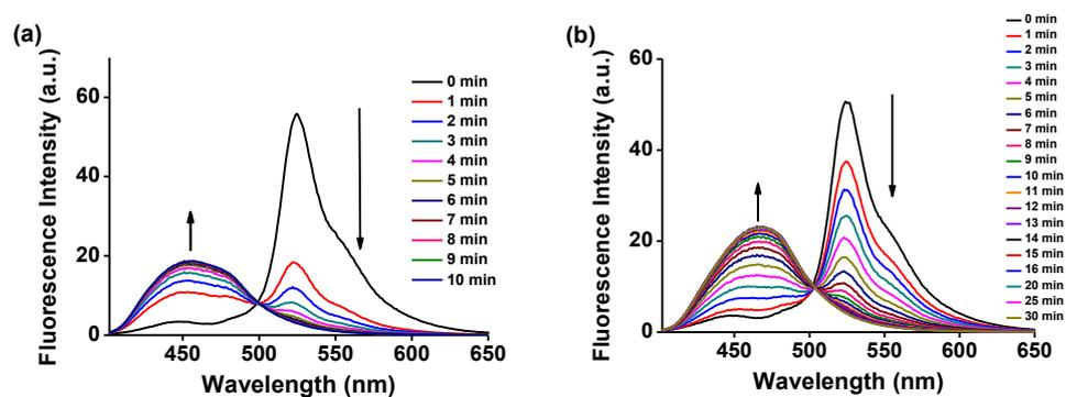
**Fig. S3** Time-dependent fluorescence spectra of the probe **1** (10  $\mu$ M) with 0.1 mM of (a) Cys and (b) Hcy. Each spectrum was acquired in HEPES buffer (pH 7.4, containing 1 %  $\text{CH}_3\text{CN}$ ) at 25  $^{\circ}\text{C}$ . Excitation wavelength is 400 nm.
