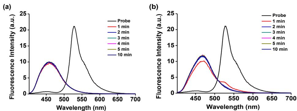
**Fig. S4** Time-dependent fluorescence spectra of the probe **1** (10  $\mu$ M) with 1.0 mM of (a) Cys and (b) Hcy. Each spectrum was acquired in HEPES buffer (pH 7.4, containing 1 %  $\text{CH}_3\text{CN}$ ) at 25  $^\circ\text{C}$ . Excitation wavelength is 400 nm.
