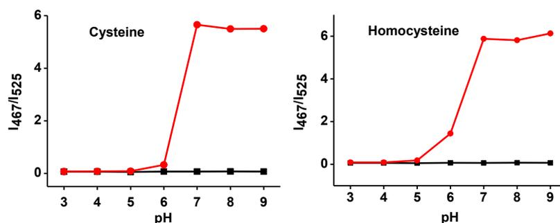
**Fig. S8** The fluorescent ratio of the probe **1** (10  $\mu$ M) at various pH value in the absence (■) or presence (●) of Cys, Hcy (0.1 mM). The spectra were recorded after incubation of the probe **1** with Cys/Hcy for 20 min at 25  $^\circ\text{C}$ . Excitation wavelength is 400 nm.
