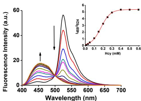
**Fig. S5** Fluorescence spectra of the probe **1** (10  $\mu$ M) upon addition of increasing concentration of Hcy. Each spectrum was acquired in HEPES buffer (pH 7.4, containing 1 %  $\text{CH}_3\text{CN}$ ) at 25  $^\circ\text{C}$ . Excitation wavelength is 400 nm.
