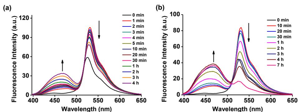
**Fig. S2** Time-dependent fluorescence spectra of the probe **1** (10  $\mu$ M) with 1.0 mM of GSH, measured at (a) 25  $^{\circ}\text{C}$  and (b) 37  $^{\circ}\text{C}$ . Each spectrum was acquired in HEPES buffer (pH 7.4, containing 1 %  $\text{CH}_3\text{CN}$ ). Excitation wavelength is 400 nm.
