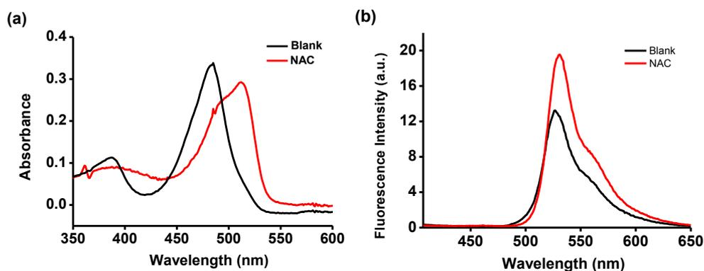
**Fig. S1** (a) Absorption and (b) emission spectrum for the reaction product between *N*-acetyl-cysteine (1.0 mM) and the probe **1** (10  $\mu$ M) in HEPES buffer (pH 7.4, containing 1 %  $\text{CH}_3\text{CN}$ ).
