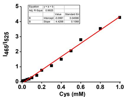
**Fig. S6** The emission ratio of the probe **1** (10  $\mu$ M) to various concentrations of Cys. The data was acquired after incubation of the probe **1** with Cys for 20 min in pH 7.4 HEPES buffer (containing 1%  $\text{CH}_3\text{CN}$ ) at 25  $^\circ\text{C}$ . Excitation wavelength is 400 nm.
