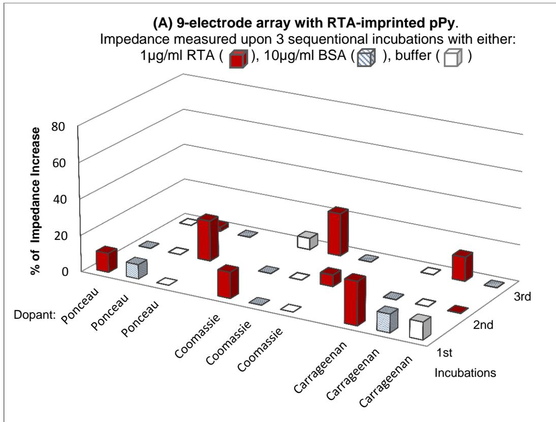
**Figure S5.** Specificity of RTA-imprinted MICP array towards RTA measured as % of Impedance increase, three consecutive incubations. pPy/ RTA-imprinted films obtained with various dopants on the array electrodes were incubated for 30 min. in either 1  $\mu$ g/ml RTA, 10  $\mu$ g/ml of BSA as nonspecific control, or binding buffer. Impedance was measured before and after the incubation. Protein binding to the MICP films calculated as % of Increase of  $-Z''$  values was plotted for each set.
