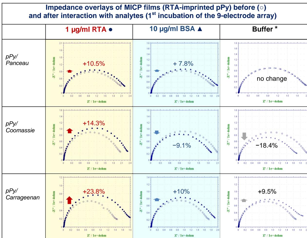
**Figure S4. AC Impedance data as overlaid Nyquist plots obtained on MICP Array.** RTA-imprinted pPy films obtained with various dopants on the array electrode were incubated for 30 min. with 1 μg/ml RTA, 10 μg/ml BSA as nonspecific control, or binding buffer. Impedance was measured before and after the incubation in the presence of 2.5 mM each Fe (II)/Fe(III) in PBS.
