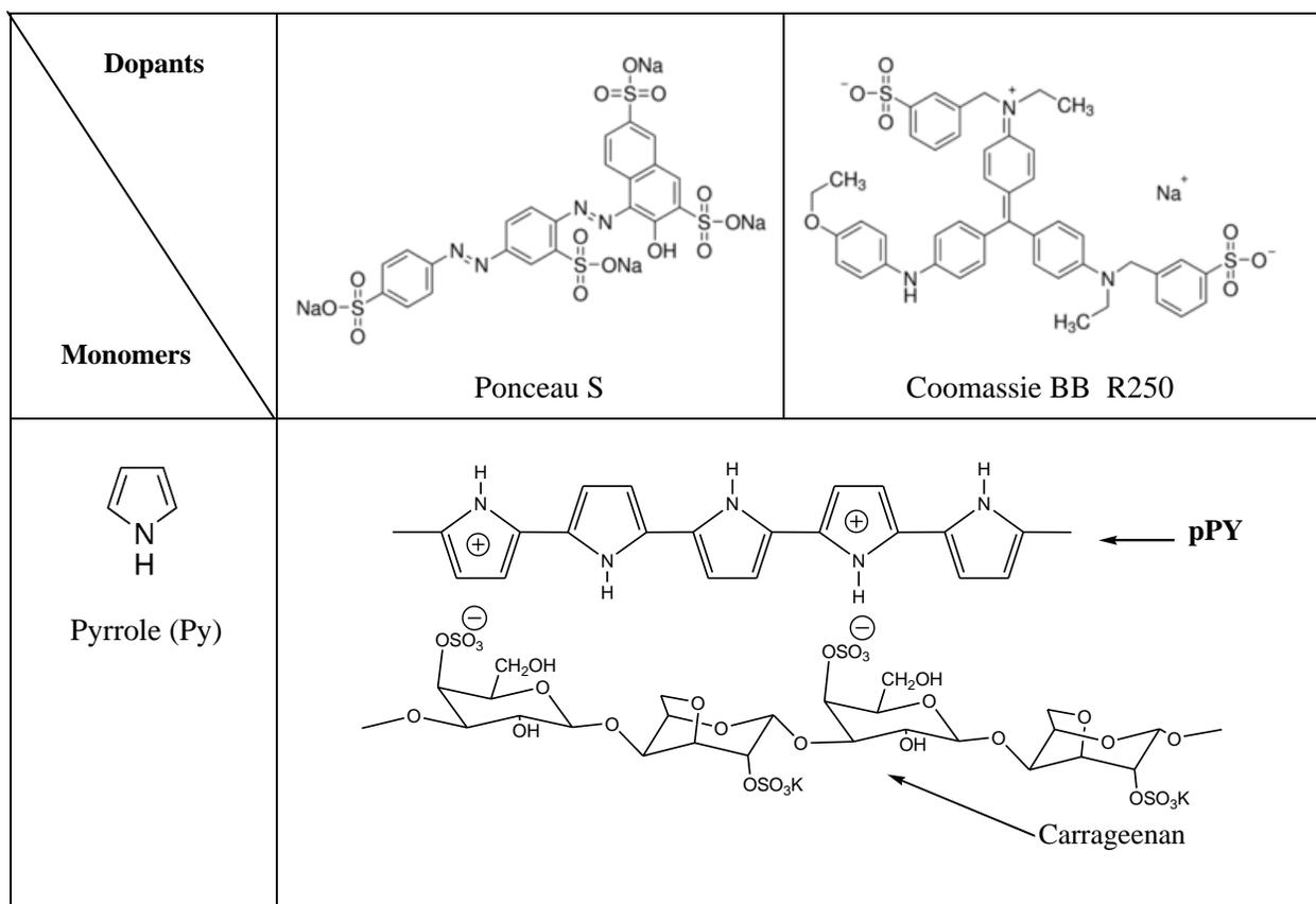
**Figure S2. Components used in MICP film preparations**
