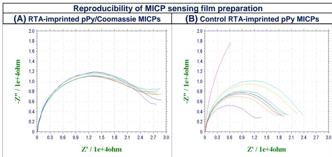
**Figure S7. Using macromolecular dopants increases MICP reproducibility.** MICP films were prepared on array electrodes in identical conditions except for Coomassie dopant. AC Impedance data as overlaid Nyquist plots obtained from **(A)** eight RTA-imprinted pPy/Coomassie MICPs and **(B)** nine RTA-imprinted pPy, all after proteinase K digestion and PBS/ Tween wash. Impedance was measured in the presence of 2.5 mM each Fe (II)/ Fe(III) in PBS.
