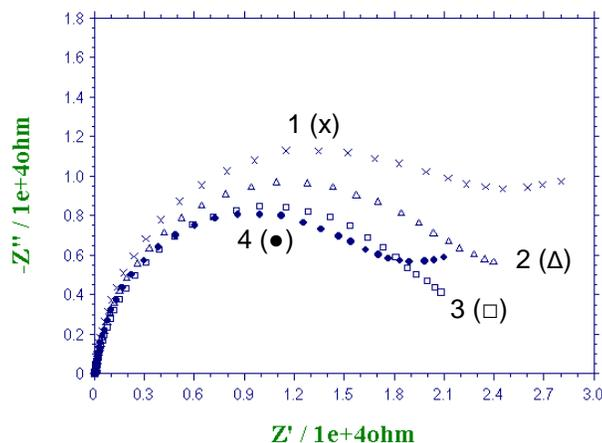
**Figure S3. Overoxidation of MICP pPy/Coomassie film imprinted with RTA.** 1: after pPy polymerization by CV; 2 and 3: two steps of overoxidation, 1 V for 1 min. each; 4: after protease treatment 2 h. and repeated PBS/SDS wash.
