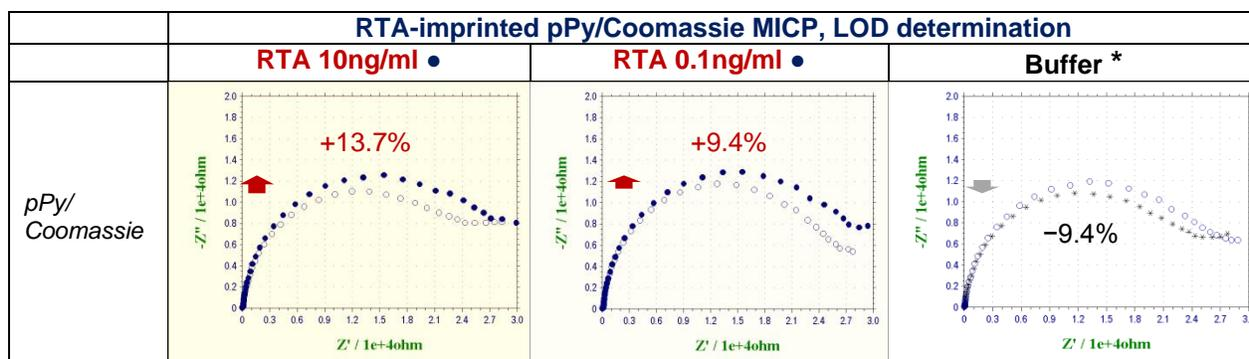
**Figure S6. LOD determination.** RTA-imprinted pPy/Coomassie films were exposed to dilutions of RTA to detect LOD. Impedance overlay before ( $\circ$ ) and after ( $\bullet$ ) exposure to 10 ng/ml and 0.1 ng/ml RTA for 30 min. AC Impedance was measured in the presence of 2.5 mM each Fe(II)/ Fe(III) in PBS. Relative Impedance increase, resulting from RTA binding was measured as % ( $\Delta Z''$ ).
