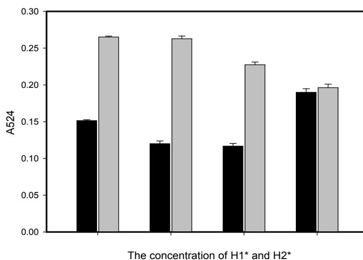
**Figure S4.** Optimization of the H1\* and H2\* concentrations. The plot shows various amounts of H1\* and H2\* vs the absorption peak of AuNPs at 524 nm with (black histogram) or without (gray histogram) 5 nM Target DNA T\*. [AuNPs] = 3 nM.
