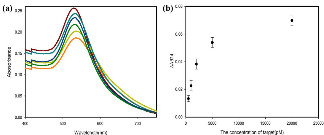
**Figure S7.** (a) UV-vis spectra detection based on CHA for different concentrations of Target T\* in 10% cell lysate. (b) UV-vis absorption peak change at 524 nm as a function of the various concentrations of T\*. [H1\*] = [H2\*] = 50 nM, [AuNPs] = 3 nM
