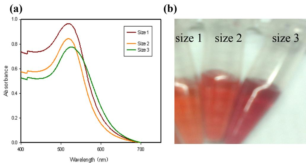
**Figure S1.** Characterization of different sized AuNPs. (a) UV absorption spectra of different sized AuNPs. (b) The visual colors of different size AuNPs.
