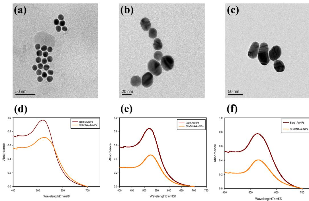
**Figure S2.** TEM images of different sizes of AuNPs: (a) size 1:  $13\pm 1$  nm; (b) size 2;  $20\pm 3$  nm; (c) size 3:  $40\pm 5$  nm. Absorption spectra of AuNPs (black line) and DNA functionalized AuNPs (red line) of (d) size 1, (e) size 2, and (f) size 3.
