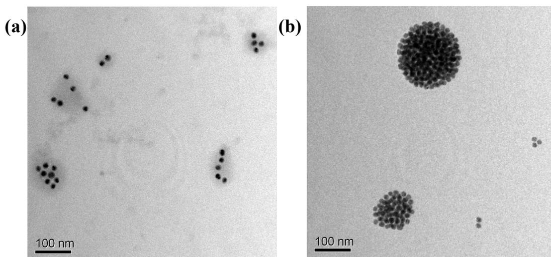
**Figure S3.** TEM images of AuNPs in HCR system without (a) or with 5 nM target DNA.
