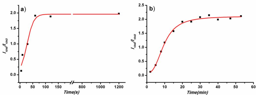
**Fig. S2** The influence of extraction time and elution time. The ratio of intensity of m/z 1040 and m/z 1043 was chosen to evaluate the degree of extraction and elution. M/z 1040 was  $[\beta\text{-}^3\text{H}]^3$ - and m/z 1043 was the double-charged ion of a synthetic phosphopeptide (MW: 2089.13 Sequence: EVVG[pS]AEAGVDAASVSEEFR). a) The effect of extraction time on ratio of intensity of m/z 1040 and m/z 1043. b) The effect of elution time on ratio of intensity of m/z 1040 and m/z 1043.
