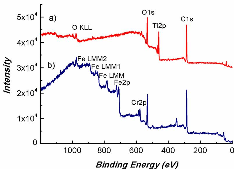
**Fig. S1** XPS characterization of stainless steel wires. a) After coated with  $\text{TiO}_2$  and b) without any pretreatment.
