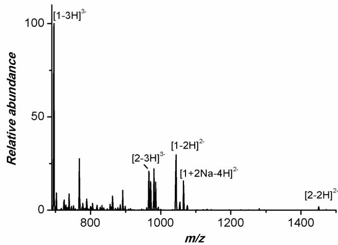
**Fig. S5** Negative ion nanoESI mass spectrum obtained after enrichment using the probe coated with TiO<sub>2</sub>. Numbers indicate the phosphopeptides obtained from the tryptic digest of egg white were listed in Table S3.
