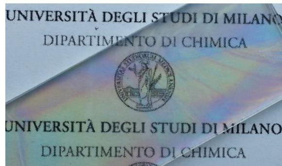
**Figure S2.** Photograph of the final device on a printed white paper with the logo of the Università degli Studi di Milano, in order to show transparency properties.
