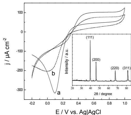
**Fig. S1.** CVs obtained at (a) FeNiPt-NRL/GC and (b) annealed FeNiPt-NRL/GC electrodes in 0.1 M PBS solution containing 1 mM  $\text{H}_2\text{O}_2$ . Potential scan rate:  $20 \text{ mV s}^{-1}$ . The inset shows the X-ray diffraction patterns of annealed FeNiPt-NRL.
