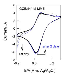
Figure S1. Cyclic voltammetric response of GCE/ $\{Nf-fc\}$ -MME in pH 7 PBS recorded at different days. Scan rate = 50 mV/s.
