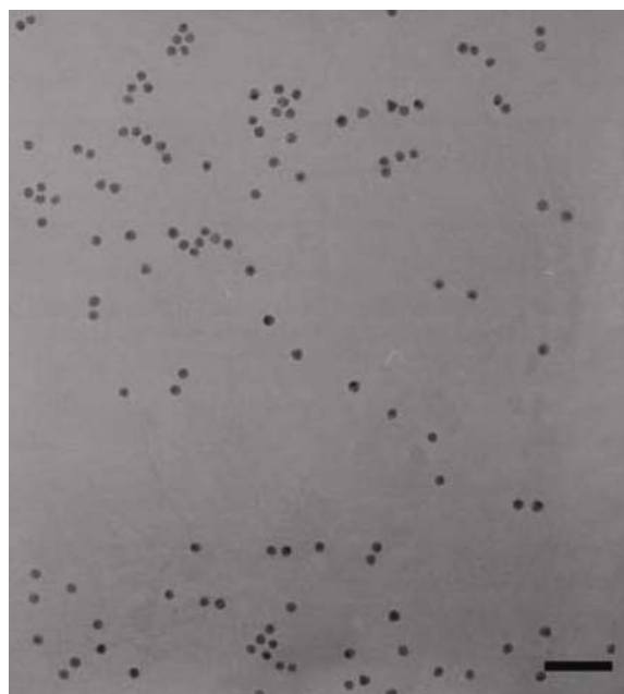
Figure 2 TEM micrograph of streptavidin-GNPs. The average size of the particles is 13 \pm 0.75 nm in diameter. The scale bar indicates 100 nm.
