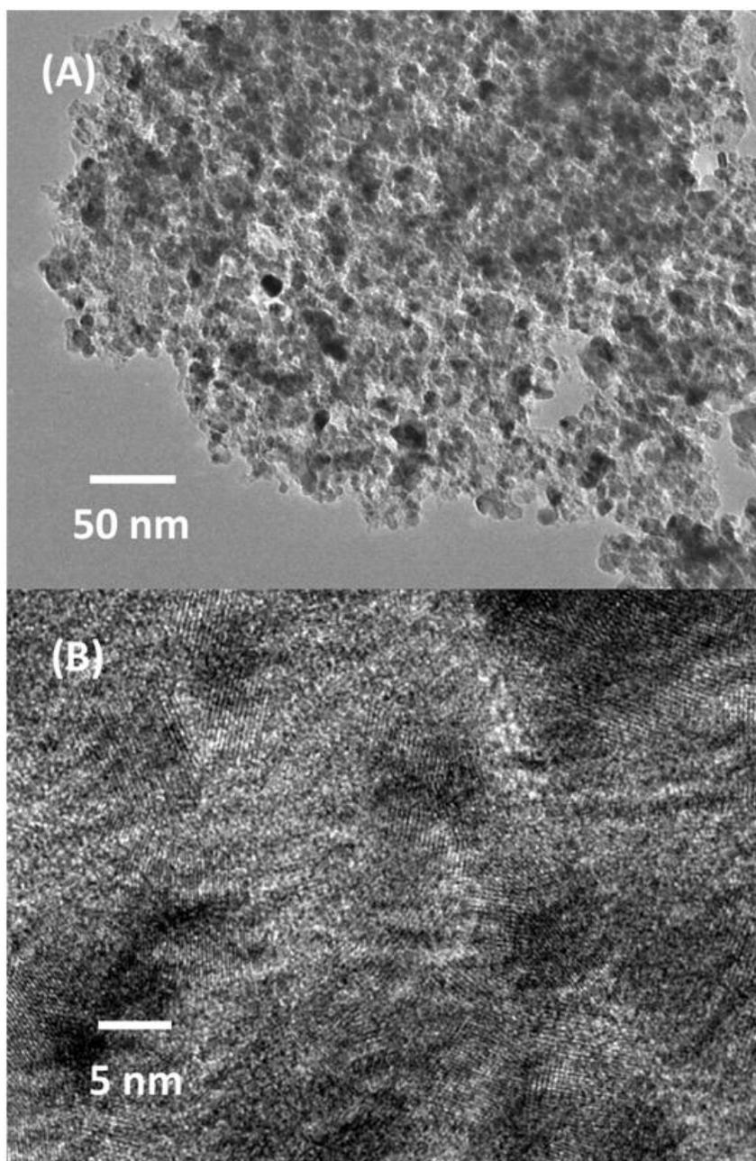
**Fig. S2.** HRTEM images [(A)- low, and (B)-high magnification] of HOM/SnO<sub>2</sub> ( $r=4.00$ ). The ordered mesoporous structure of monolith was destroyed when the SnO<sub>2</sub> content was increased to 80%. The monolith contains the aggregated SnO<sub>2</sub> nanocrystals with an average of about 5 nm.
