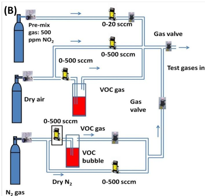
**Fig. S1.** Schematic diagram of gas-sensing measurement system. (A) The electrical current and resistance of sensors are automatically measured using a Digital Source Meter (Keithley model 2400) controlled by PC computer via IEEE cable and Labview program. (B) Schematic diagram of the VOC bubbler system.
