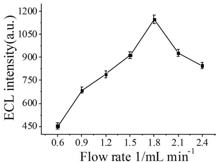
Figure S.4 Effect of pump 1 on |ECL intensity
