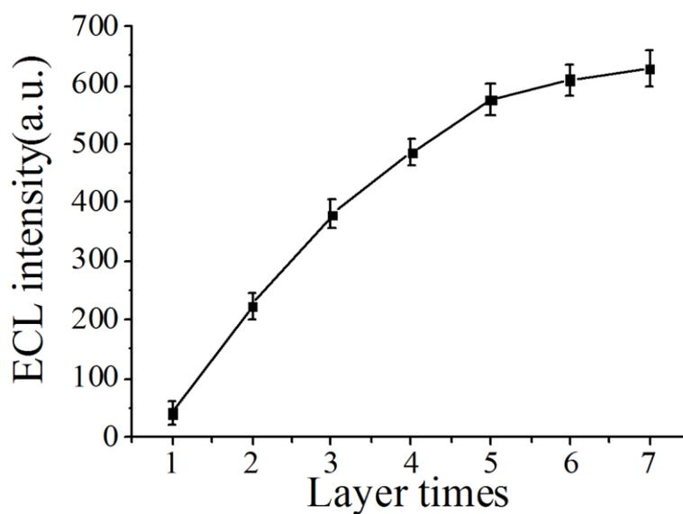
Figure S.2 Effect of layer times on ECL intensity
