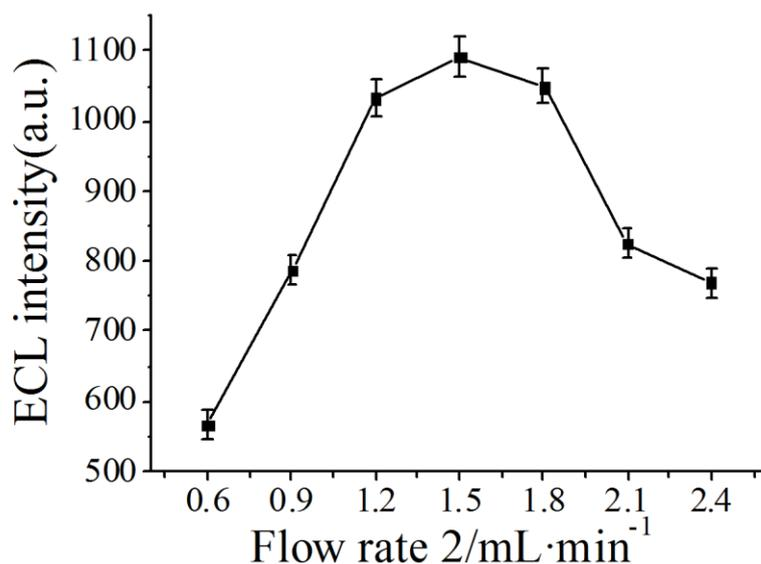
Figure S.5 Effect of pump 2 on ECL intensity
