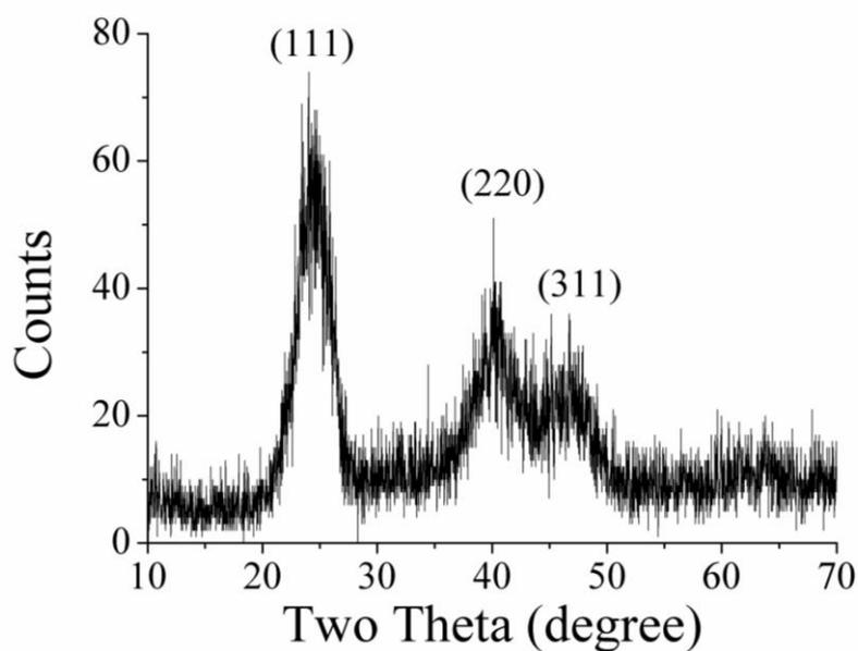
Figure S.1.3 XRD pattern of CdTe
