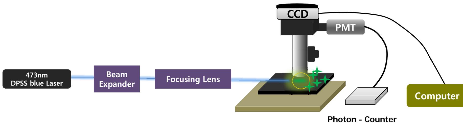
**Schematic of Lab-built LIF (Laser Induced Fluorescence) Microscope System**
