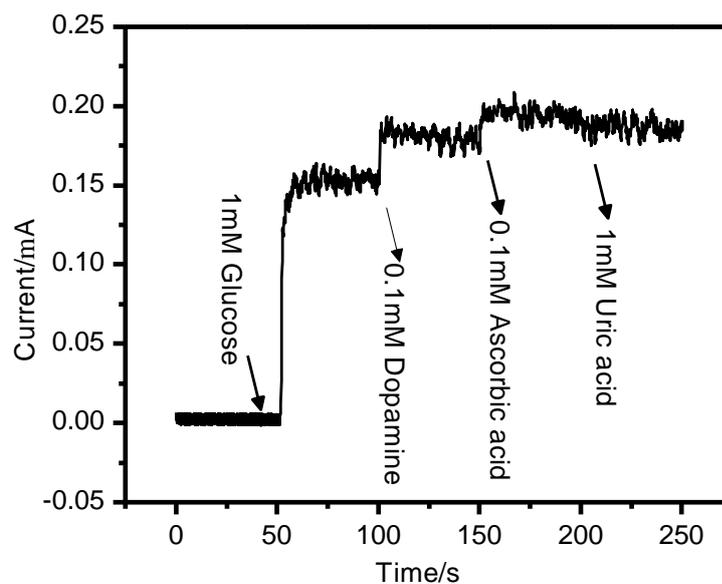
Fig. 3 Amperometric response to injection of 1 mM glucose, 0.1 mM dopamine, 0.1 mM ascorbic acid and 1 mM uric acid
