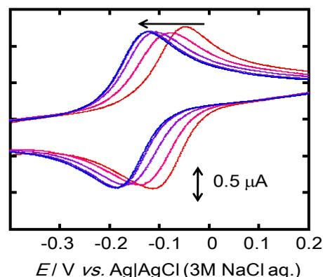
Fig. S1 The shifts of cyclic voltammogram of [Ru<sup>II</sup>(acac)<sub>2</sub>(4-Bpy)(4-Cpy)] measured after 5 min from the addition of G2 dendrimer (0, 0.25, 0.50, 0.75, 1.00, 1.25 eq.) in 0.1 mol dm<sup>-3</sup> NaClO<sub>4</sub>/(H<sub>2</sub>O:MeOH = 8:2) at GCDE ( $\phi = 3$  mm) at 25 °C. Scan rate = 100 mV s<sup>-1</sup>.
