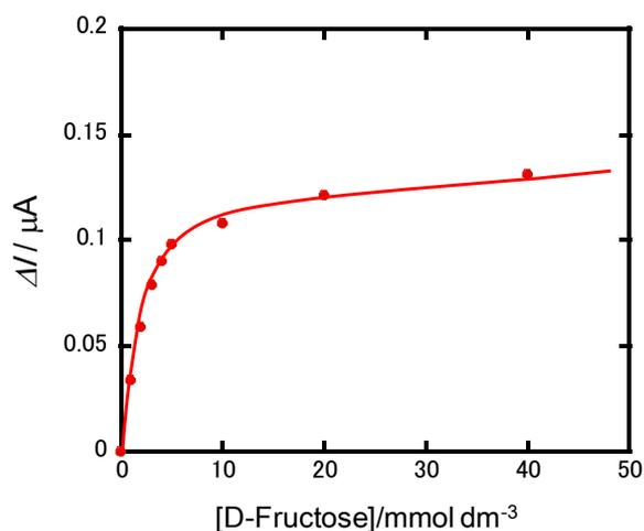
Fig. S5 The peak current shifts of DPV of  $[\text{Ru}^{\text{II}}(\text{acac})_2(4\text{-Bpy})(4\text{-Cpy})]$  containing one equivalent G2 dendrimer by the addition of D-fructose.
