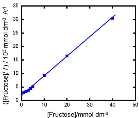
Fig. S6 The plot of  $([\text{Fructose}]/I)$  vs.  $[\text{Fructose}]$   $[\text{Ru}^{\text{II}}(\text{acac})_2(4\text{-Bpy})(4\text{-Cpy})]$ /dendrimer complex.  $I$  is the peak current of DPV.
