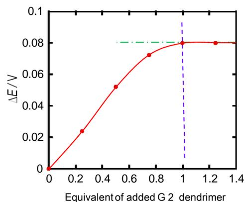
Fig. S2 The peak potential shifts of DPV of [Ru<sup>II</sup>(acac)<sub>2</sub>(4-Bpy)(4-Cpy)] measured after 5 min from the addition of G2 dendrimer in 0.1 mol dm<sup>-3</sup> NaClO<sub>4</sub>/(H<sub>2</sub>O:MeOH = 8:2) at GCDE ( $\phi = 3$  mm) at 25 °C.
