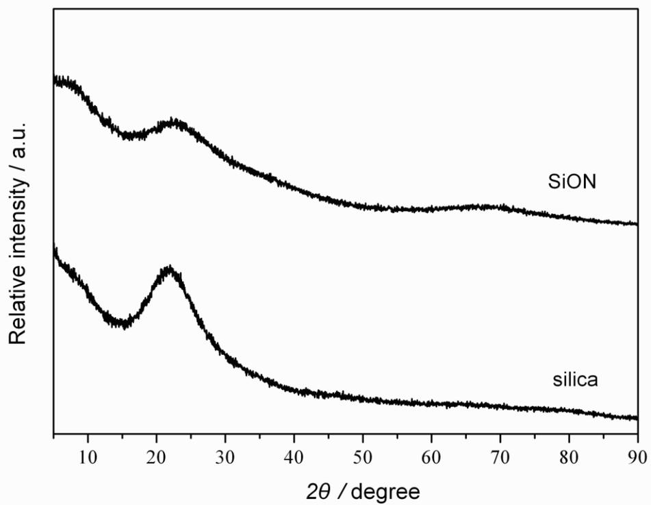
**Fig. S1** XRD patterns of parent silica and sph-SiON.
