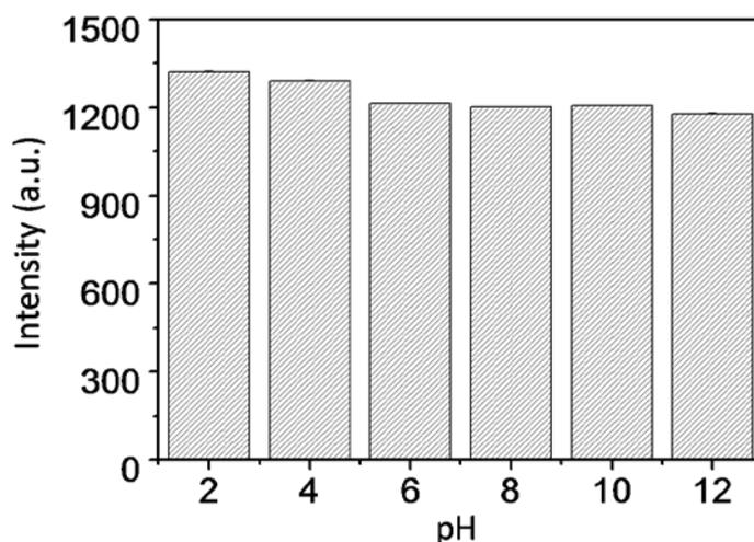
**Fig. S1** Effect of pH on the fluorescence intensity at 437 nm of chemosensor **1** ( $5 \times 10^{-6}$  M) in 100% aqueous solution. The pH values of the solution were adjusted by very small amount of HCl and KOH aqueous solution.
