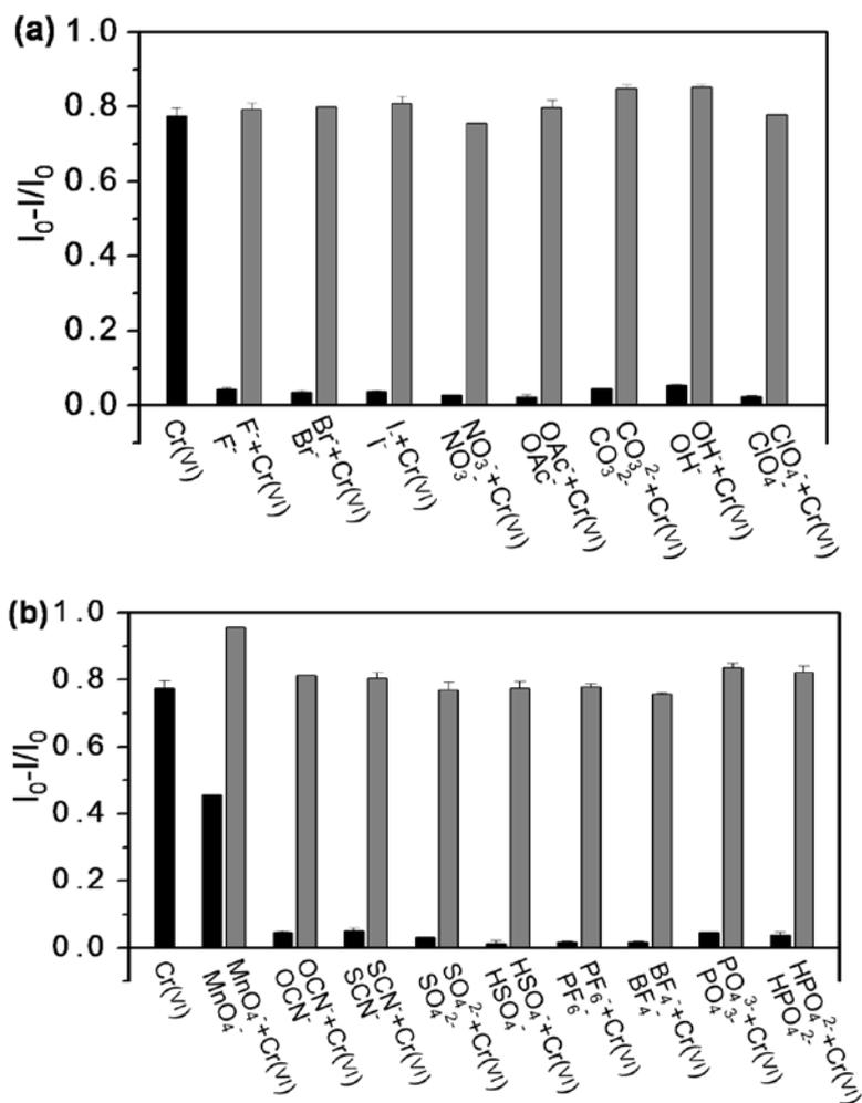
**Fig. S9** Quenching rate at 437 nm of  $5 \times 10^{-6}$  M chemosensor **1** in aqueous solution at pH = 4.0. Dark bars represent the addition of 100 equiv. of anions, and gray bars represent the subsequent addition of 100 equiv. of Cr(VI) to the solution.
