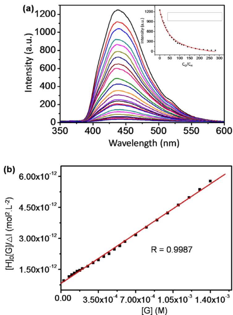
**Fig. S3** (a) Fluorescence titration spectra of chemosensor **1** ( $5 \times 10^{-6}$  M) upon addition of different equiv. of Cr(VI) (0 - 280 equiv.) in 100% aqueous solution at pH 4.0. Inset: fluorescence intensity development with the increasing equiv. of Cr(VI). (b) Plot of  $[H]_0[G]/\Delta I$  versus  $[G]$  for calculating the inner filter constant of chemosensor **1** with Cr(VI) in 100% aqueous solution at pH 4.0.
