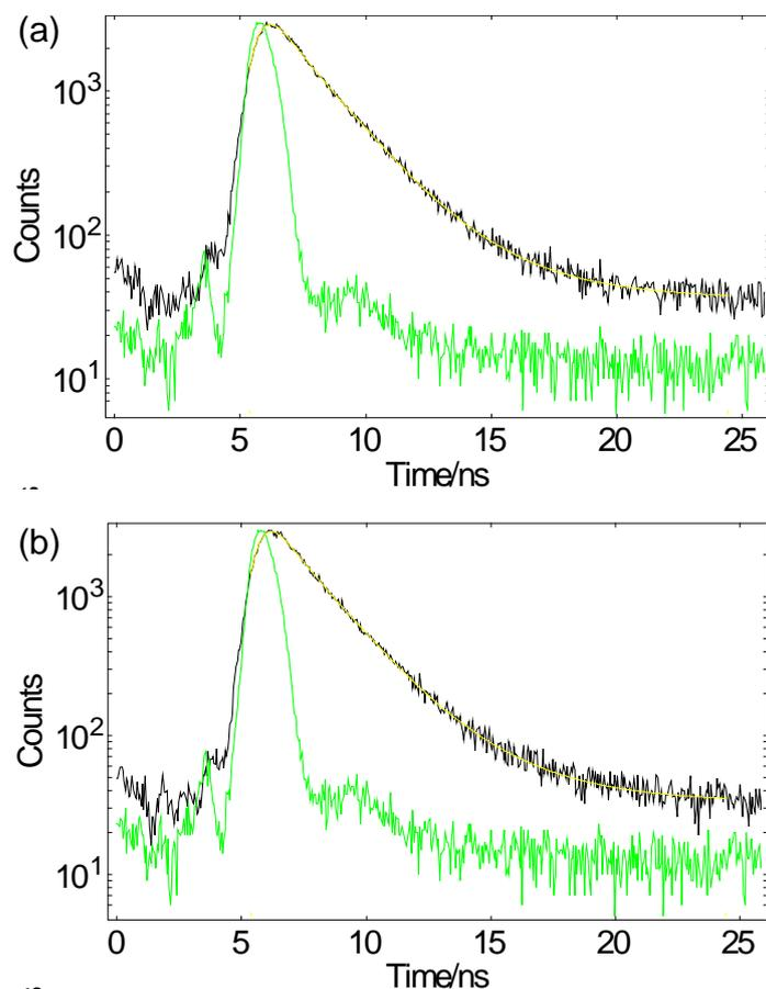
**Fig. S5** (a) Fluorescence decay curve of the chemosensor **1** ( $5 \times 10^{-6}$  M) in the absence of Cr(VI). (b) Fluorescence decay curve of chemosensor **1** ( $5 \times 10^{-6}$  M) in the presence of 100 equiv. of Cr(VI). The decay curves were fitted to the biexponential function with acceptable  $\chi^2$  (1.2 and 1.1 respectively).
