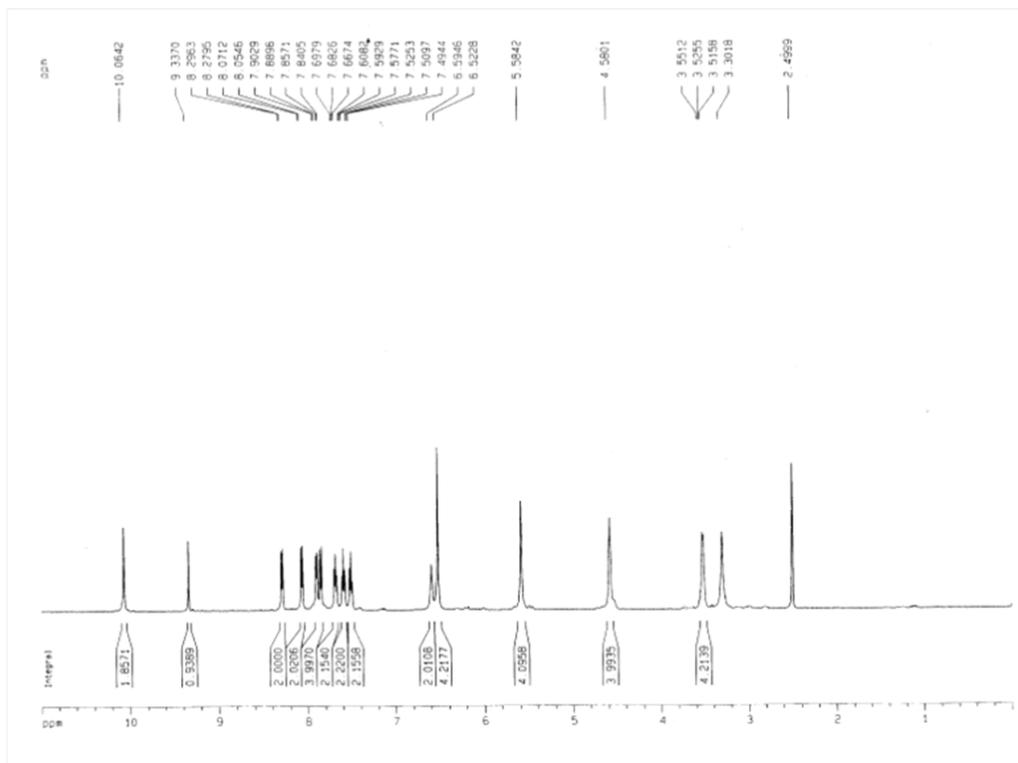
Fig. S11  $^1\text{H}$  NMR of chemosensor **1** in  $\text{DMSO-d}_6$ .
