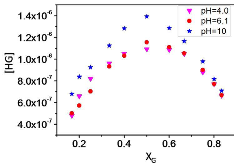
**Fig. S7** Fluorescence Job's plot of chemosensor **1** with Cr(vi) in 100% aqueous solution at pH 4.0 (▼), 6.1(●) and 10 (★) respectively, where [G]+[H] = 5 × 10<sup>-6</sup> M.
