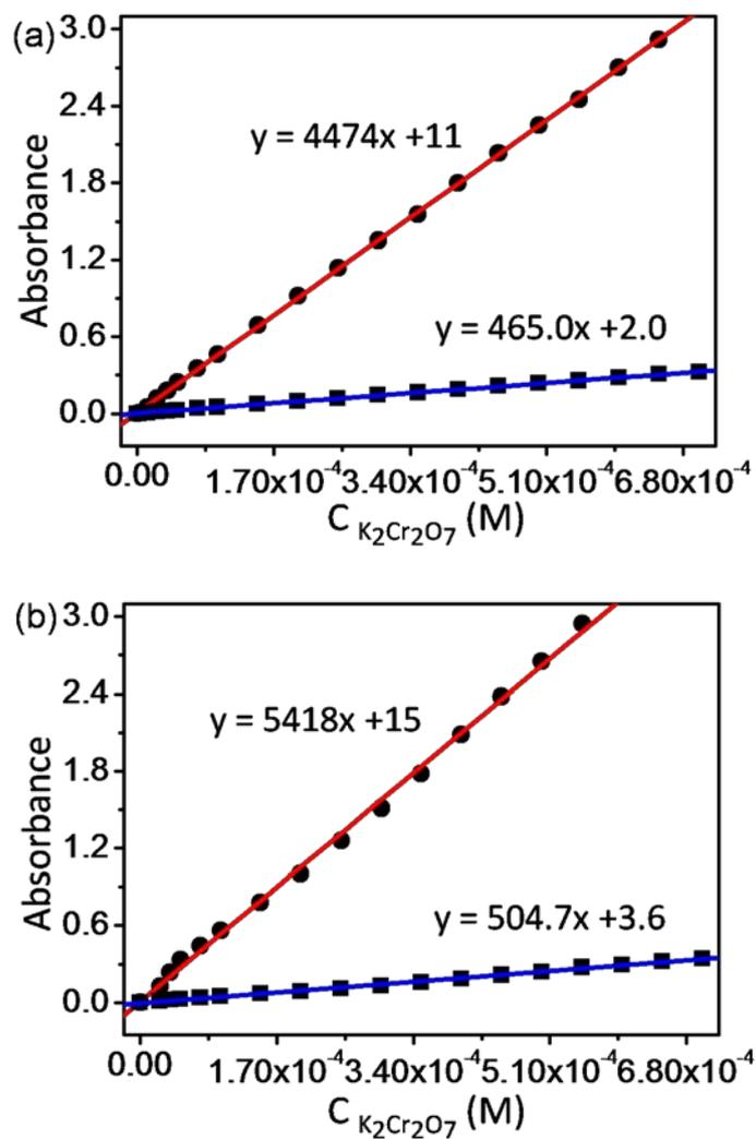
**Fig. S2** Calculation of the extinction coefficients of  $K_2Cr_2O_7$  at 259 nm (red lines) and 437 nm (blue lines) in water (a) and in 98% MeCN aqueous solution (b) respectively.
