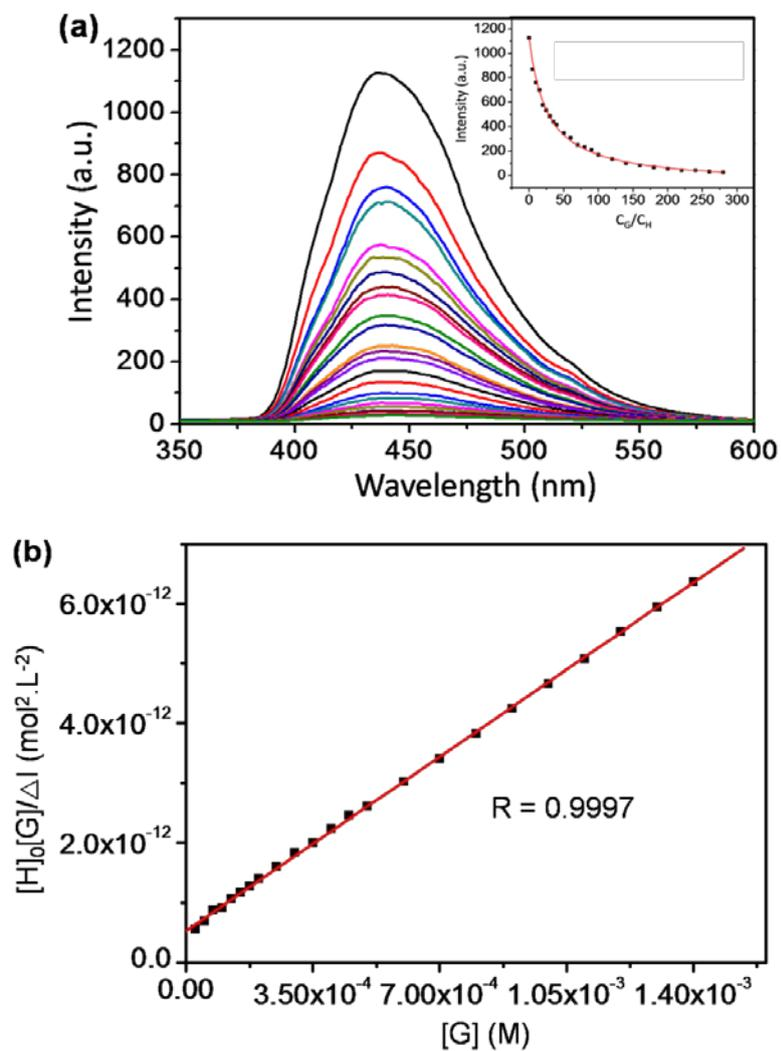
**Fig. S4** (a) Fluorescence titration spectra of chemosensor **1** ( $5 \times 10^{-6}$  M) upon addition of different equiv. of Cr(vi) (0 - 280 equiv.) in 100% aqueous solution at pH 10. Inset: fluorescence intensity development with the increasing equiv. of Cr(vi). (b) Plot of  $[H]_0[G]/\Delta I$  versus  $[G]$  for calculating the inner filter constant of chemosensor **1** with Cr(vi) in 100% aqueous solution at pH 10.
