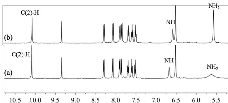
**Fig. S6** Partial <sup>1</sup>H NMR spectra of chemosensor **1** (10 mM) in the absence (a) and presence (b) of Cr(vi) (1 equiv.) in DMSO-d<sub>6</sub>.
