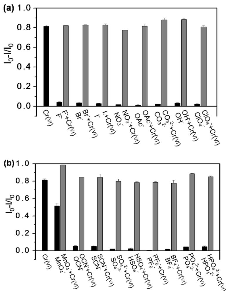
**Fig. S10** Quenching rate at 437 nm of  $5 \times 10^{-6}$  M chemosensor **1** in aqueous solution at pH = 10. Dark bars represent the addition of 100 equiv. of anions, and gray bars represent the subsequent addition of 100 equiv. of Cr(VI) to the solution.
