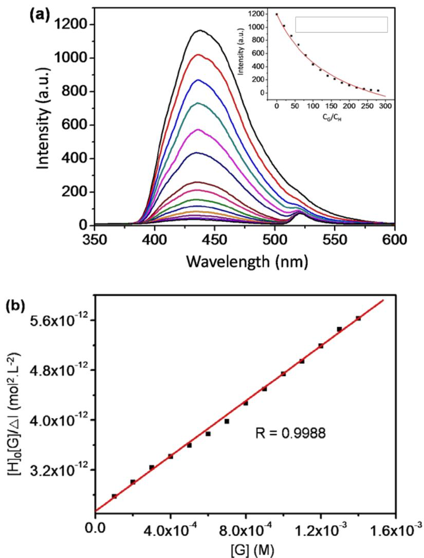
**Fig. S8** (a) Fluorescence titration spectra of chemosensor **1** ( $5 \times 10^{-6}$  M) upon addition of different equiv. of  $\text{MnO}_4^-$  (0 - 280 equiv.) in 100% aqueous solution at pH 6.1. Inset: fluorescence intensity development with the increasing equiv. of  $\text{MnO}_4^-$ . (b) Plot of  $[\text{H}]_0[\text{G}]/\Delta I$  versus  $[\text{G}]$  for calculating the inner filter constant of chemosensor **1** with  $\text{MnO}_4^-$  in 100% aqueous solution at pH 6.1.
