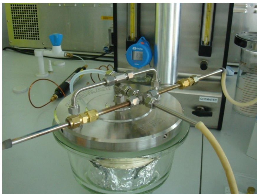
Fig. S2 Picture of foam sealant sample being tested under FLEC
