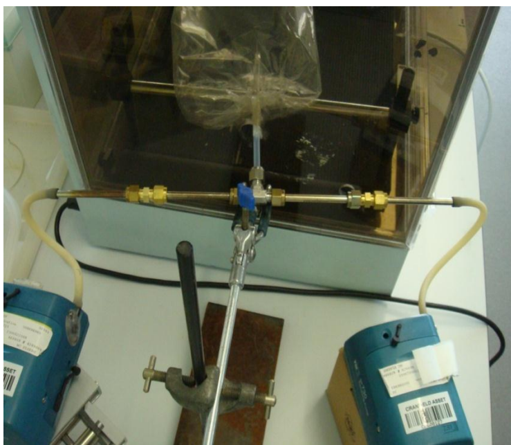
Fig. S4 Picture of experimental set up for Nalophan bag tests
