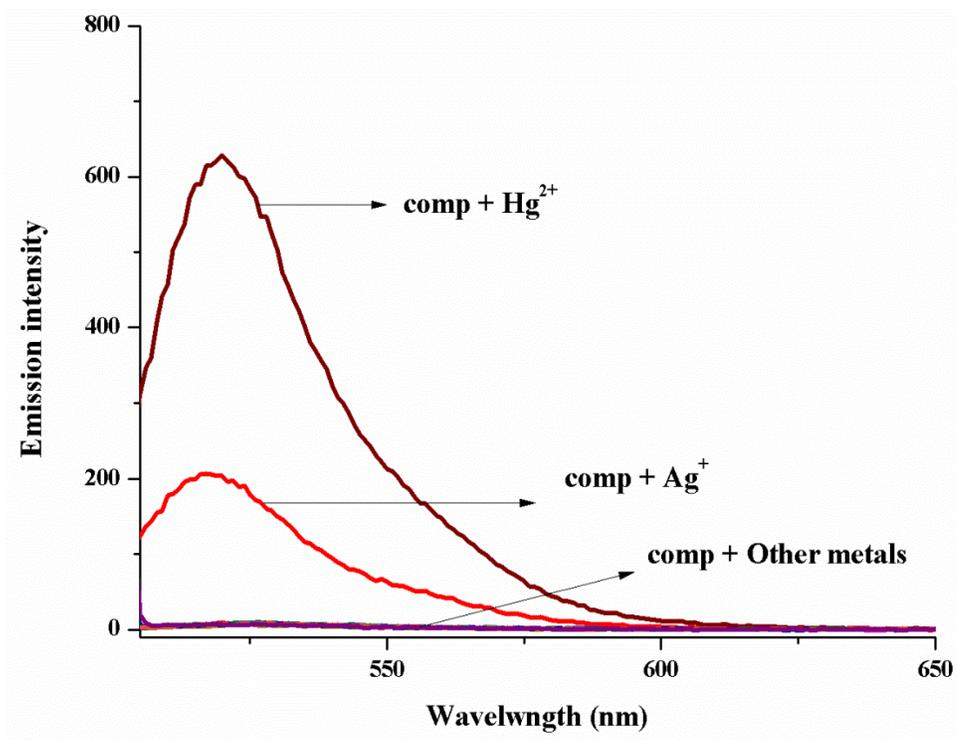
**Fig. S8:** Emission spectra of compound **1** ( $5 \times 10^{-6}$  M, buffered H<sub>2</sub>O: DMSO 80:20; pH 7.4; buffer<sub>aq</sub>: 20 mM HEPES) with Ca<sup>2+</sup>, Cd<sup>2+</sup>, Co<sup>2+</sup>, Cu<sup>2+</sup>, Fe<sup>2+</sup>, Mg<sup>2+</sup>, Mn<sup>2+</sup>, Pb<sup>2+</sup>, Zn<sup>2+</sup>, Ni<sup>2+</sup>, Ag<sup>+</sup> and Hg<sup>2+</sup> ( $3.33 \times 10^{-3}$  M in water) incubated for 30 min at RT.  $\lambda_{exc}$  = 490 nm.
