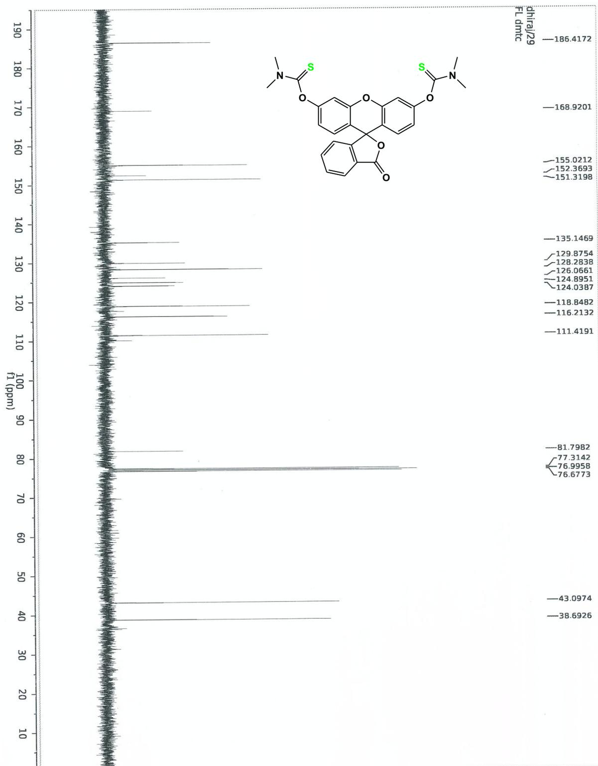
Fig. S2:  $^{13}\text{C}$  NMR spectrum of compound 1.
