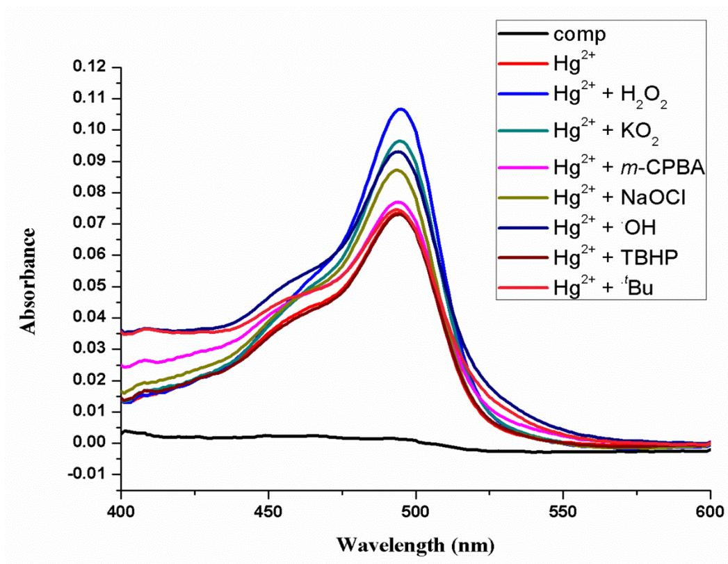
**Fig. S10:** Absorption spectra of compound **1** ( $5 \times 10^{-6}$  M, buffered H<sub>2</sub>O: DMSO 80:20; pH 7.4; buffer<sub>aq</sub>: 20 mM HEPES) with Hg<sup>2+</sup> (10 μL 0.1 M in water) incubated for 30 min at RT and different ROS ( $3.33 \times 10^{-3}$  M in water) 30 min. at RT.  $\lambda_{exc} = 490$  nm.
