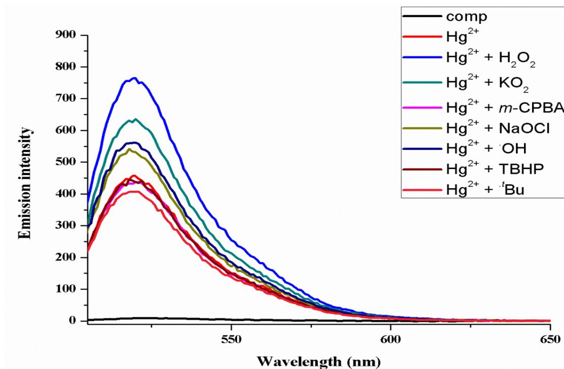
**Fig. S9:** Emission spectra of compound **1** ( $5 \times 10^{-6}$  M, buffered H<sub>2</sub>O: DMSO 80:20; pH 7.4; buffer<sub>aq</sub>: 20 mM HEPES) with Hg<sup>2+</sup> ( $3.33 \times 10^{-3}$  M in water) incubated for 30 min at RT and different ROS ( $3.33 \times 10^{-3}$  M in water) 30 min. at RT.  $\lambda_{exci} = 490$  nm.
