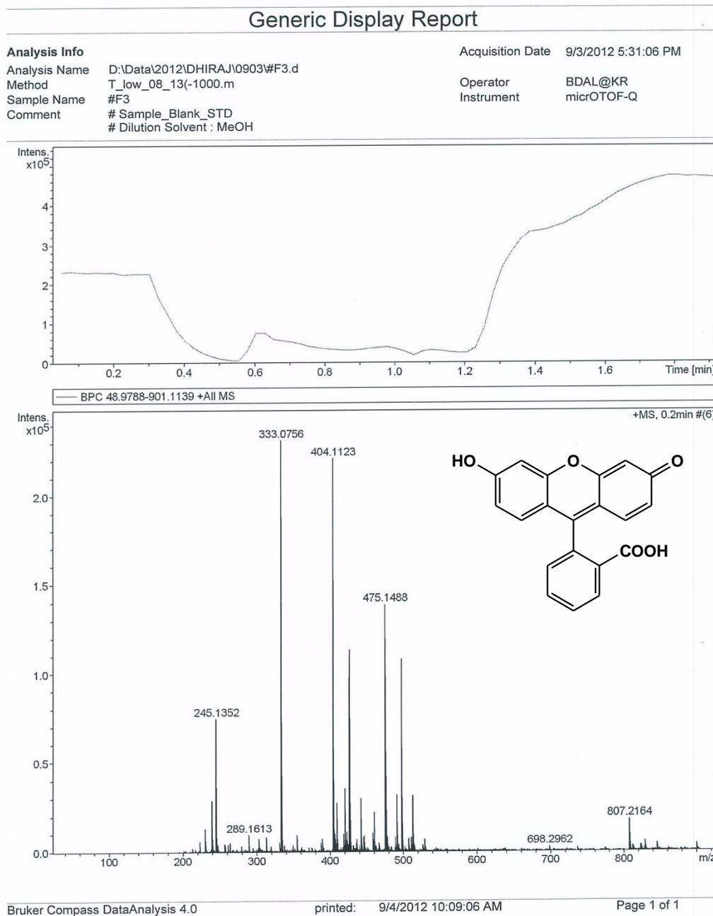
**Fig. S7:** ESI – mass spectrum of compound **1** +  $\text{Hg}^{2+}$  +  $\text{H}_2\text{O}_2$ .
