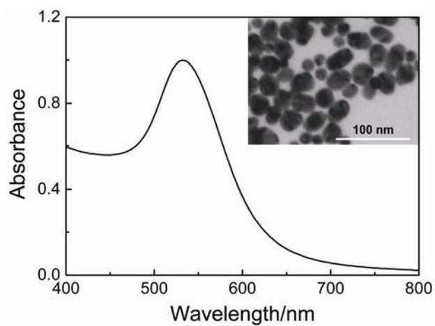
**Fig. S1** TEM micrograph (inset) and corresponding UV-visible spectrum of GNP probes. The average size of GNP probes is  $30 \pm 5$  nm.
