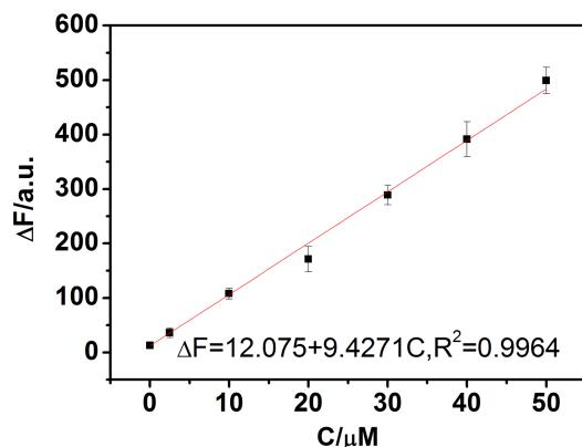
Fig. S4 Plots of absolute changes of the fluorescence intensity of C-dots at 410 nm versus the concentration of choline.
