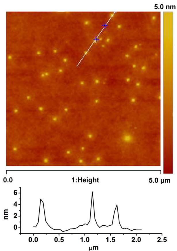
Fig. S1 AFM of C-dots
