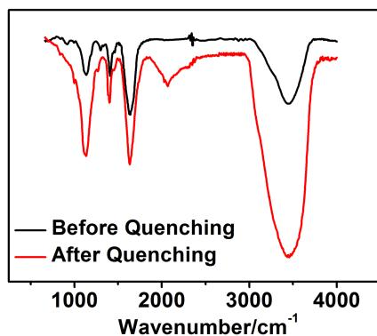
Fig. S3 FTIR of C-dots before and after quenching by  $\text{Fe}^{2+}$  and  $\text{H}_2\text{O}_2$
