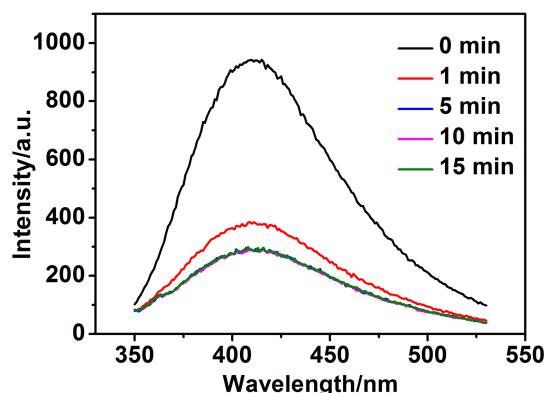
Fig. S2 Time-dependent fluorescence changes of C-dots in the presence of  $\text{H}_2\text{O}_2$  (100  $\mu\text{M}$ ) and  $\text{Fe}^{2+}$  (0.34 mM)
