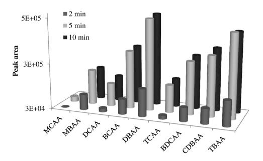
Fig. S2 Influence of the sonication time on the extraction efficiency (as peak area) of the back-microextraction when using isopropyl ether (100  $\mu$ L). The spiked concentrations of HAAs were 5 mg·L<sup>-1</sup>.
