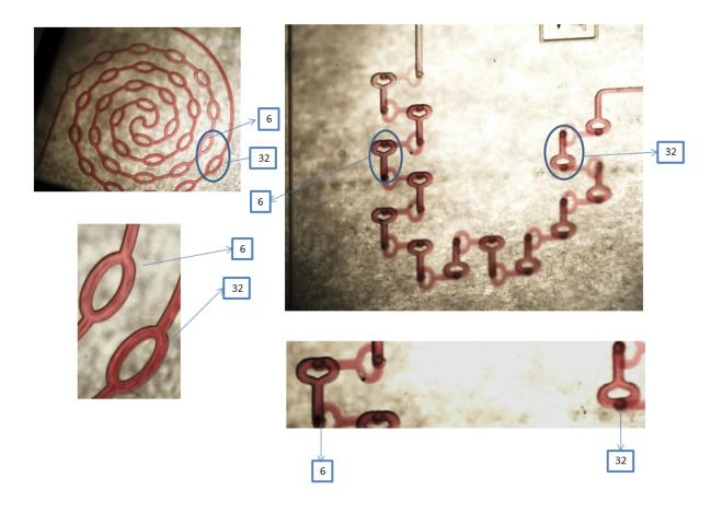
**Supplement 1:** Left top and bottom: mixing in flow splitting unit numbers 6 and 32; a difference in colour can be observed. The colour of the solution in unit 6 is lighter than that in unit 32, indicating that the mixing was incomplete in unit 6. Right top and bottom: mixing in flow splitting unit numbers 6 and 26. Differences in colour can be observed. The colour of the solution in unit 6 is the same as that in unit 32, indicating that the mixing was complete in unit 6.
