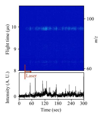
Figure S1 Two-dimensional display for a microemulsion obtained using a pair of concentric capillaries where the inner diameters of the inner and outer capillaries were 50 and 200  $\mu$ m, respectively. The time course of the peak area of toluene ion is also shown. Concentration: 400 ng/ $\mu$ L for toluene, 6,600 ng/ $\mu$ L for SDS, and 3,000 ng/ $\mu$ L for 1-pentanol.
