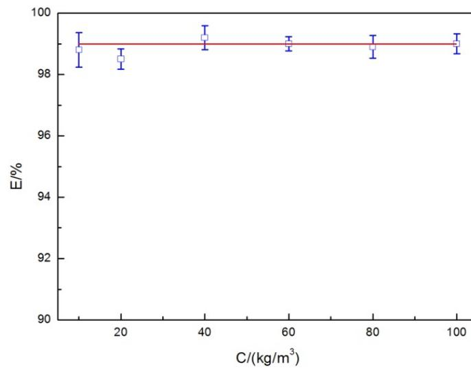
Separation efficiency of hydrocyclone under different feed rate of FPAPs
