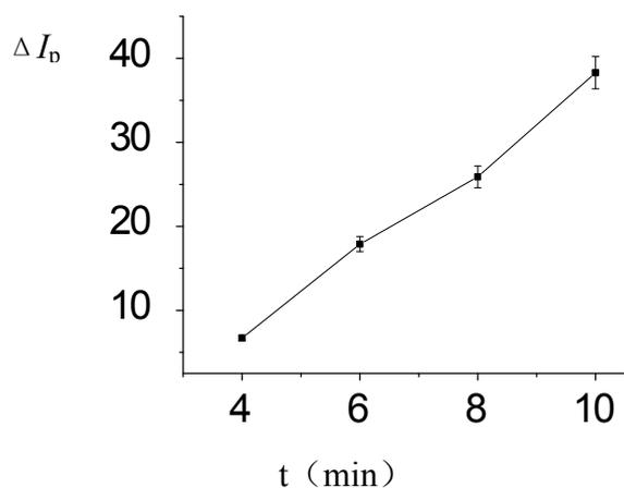
**Fig. 7 S** Effect of reaction time on the  $\Delta I_p$  of the system (when the reaction time was 4, 6, 8, 10 min, corresponding the  $\Delta I_p$  of the system was 8.7, 17.9, 25.9, 36.3, respectively.)
