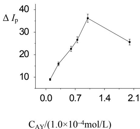
**Fig. 1 S** Effect of concentration of AY on the  $\Delta I_p$  of the system (when the concentrations of AY were 0, 0.1, 0.3, 0.75, 1.0, 2.0 ( $\times 10^{-4}$ ), corresponding the  $\Delta I_p$  of the system was 9.0, 15.9, 22.6, 28.6, 36.2, 25.6, respectively.)
