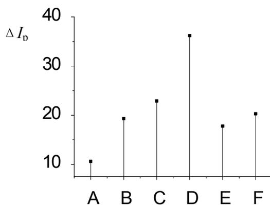
**Fig. 11 S** Effect of oxidants on the  $\Delta I_p$  of the system (when the oxidants were  $\text{KClO}_3$  (A),  $\text{K}_2\text{S}_2\text{O}_8$  (B),  $\text{KIO}_4$  (C),  $\text{H}_2\text{O}_2$  (D),  $\text{NaIO}_4$  (E) and  $(\text{NH}_4)_2\text{S}_2\text{O}_8$  (F), corresponding the  $\Delta I_p$  of the system was 10.6, 19.3, 22.9, 36.2, 17.8, 20.3, respectively.)
