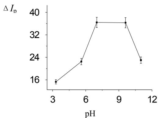
**Fig. 9 S** Effect of pH values on the  $\Delta I_p$  of the system (when the pH values were 3.30, 5.60, 7.00, 9.60, 11.0, corresponding the  $\Delta I_p$  of the system was 15.3, 22.5, 36.4, 36.3, 23.0, respectively.)
