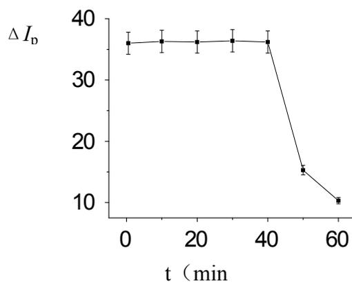
**Fig.10 S** Effect of time on the stability of the system (when the standing time was 0, 5, 10, 20, 30, 40, 50, 60 min, corresponding the  $\Delta I_p$  of the system was 36.0, 36.3, 36.2, 36.4, 36.1, 36.2, 15.3, 10.3, respectively.)
