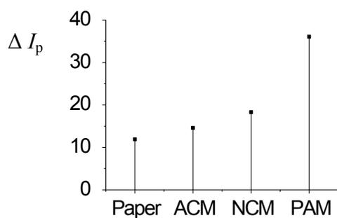
**Fig. 5 S** Effect of solid substrate on the  $\Delta I_p$  of the system (when the solid substrates were paper, PAM, ACM, PAM, corresponding the  $\Delta I_p$  of the system was 11.9, 14.6, 18.3, 36.1, respectively.)
