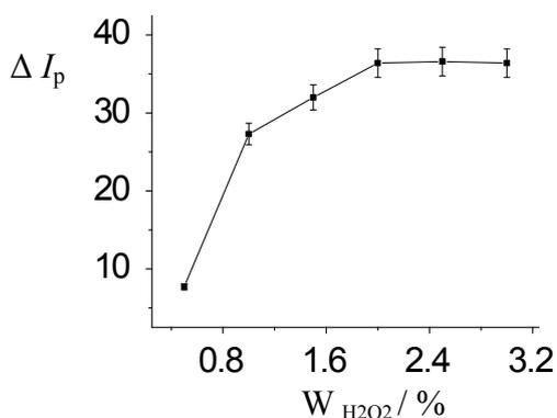
**Fig. 3 S** Effect of concentration of  $H_2O_2$  on the  $\Delta I_p$  of the system (when the concentrations of  $H_2O_2$  were 0.5, 1.0, 1.5, 2.0, 2.5, 3.0%, corresponding the  $\Delta I_p$  of the system was 7.7, 27.3, 32.0, 36.4, 36.6, 36.4, respectively.)
