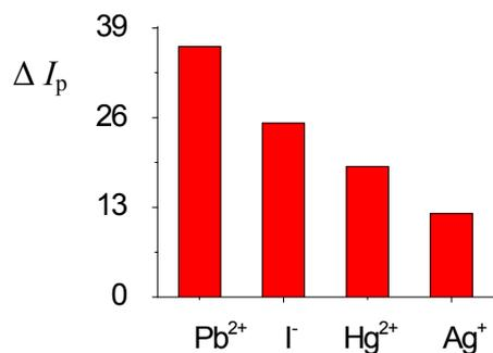
**Fig. 6 S** Effect of ion perturber on the  $\Delta I_p$  of the system (when the ion perturbers were  $Pb^{2+}$ ,  $I^-$ ,  $Hg^{2+}$ ,  $Ag^+$ , corresponding the  $\Delta I_p$  of the system was 36.3, 25.2, 18.9, 12.1, respectively.)
