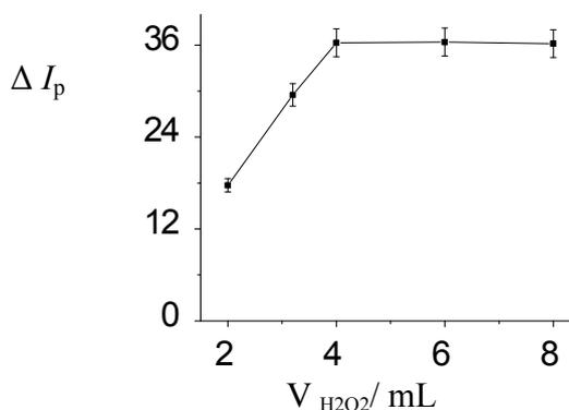
**Fig. 4 S** Effect of dosage of  $H_2O_2$  on the  $\Delta I_p$  of the system (when the dosages of  $H_2O_2$  were 2.00, 3.20, 4.00, 6.00, 8.00 mL, corresponding the  $\Delta I_p$  of the system was 17.7, 29.5, 36.3, 36.4, 36.2, respectively.)
