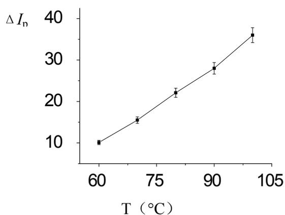
**Fig. 8 S** Effect of reaction temperature on the  $\Delta I_p$  of the system (when the reaction temperature was 60, 70, 80, 90, 100 °C, corresponding the  $\Delta I_p$  of the system was 10.1, 15.5, 22.1, 28.0, 36.0, respectively.)
