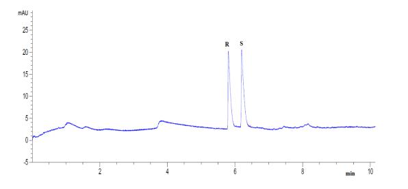
**Figure 1S.** Electropherogram of the chiral separation of CIT. Experimental conditions: capillary: 60 cm (50 cm effective length) 50 mm id; detection: 214 nm; applied voltage: 18 kV; temperature: 20  $^{\circ}$ C; injection: 60 mbar 5 s; separation solution: 50 mM phosphate buffer pH 5.0 containing 15.0% (w/v) MD with DE 4-7 as chiral selector.
