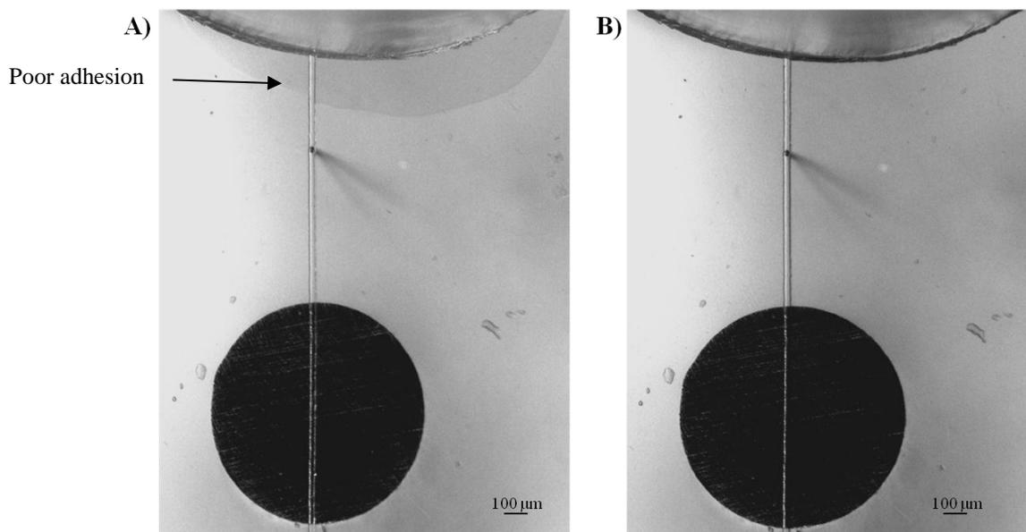
**Figure S-1.** Improvement of PDMS-PS adhesion with chlorotrimethylsilane stamping. **A)** Untreated PDMS is sealed on PS over embedded electrodes. **B)** The PDMS is stamped with chlorotrimethylsilane for one hour and then sealed onto the PS base with embedded electrodes. The PDMS microchip exhibits improved adhesion and full sealing around the sample waste reservoir after the chlorotrimethylsilane stamping method is performed.
