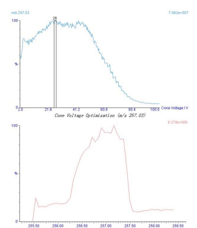
Optimized MS Spectrum (at Cone Voltage 26V)
