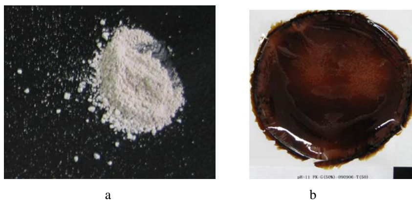
Figure 1. The photographs of chicken feather keratin powder(a) and keratin film(b) .
