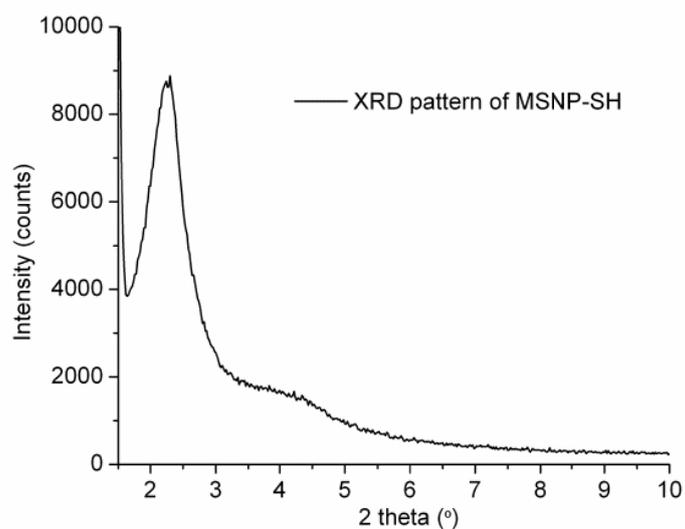
**Figure S2.** Powder X-ray diffraction pattern of MSNP-SH.
