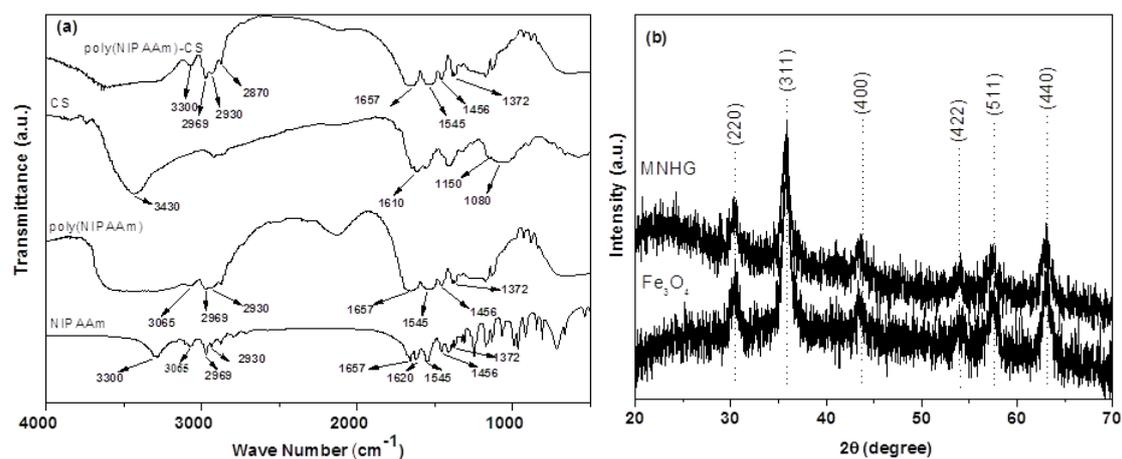
**Fig. S1.** (a) FT-IR spectra of poly(NIPAAm)-CS composite along with NIPAAm monomer indicating polymerization of NIPAAm as well as its grafting with chitosan (CS). (b) X-ray diffraction pattern of MNHG along with  $\text{Fe}_3\text{O}_4$  NPs showing confirmation of presence of NPs into it as all the peaks indexed for magnetite are present in the MNHG as well.
