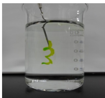
Figure R1. Photographs of thermo-gelation for P 3k 3L0.9 solution in PBS (pH 7.4, 140 mM) at 37 °C.
