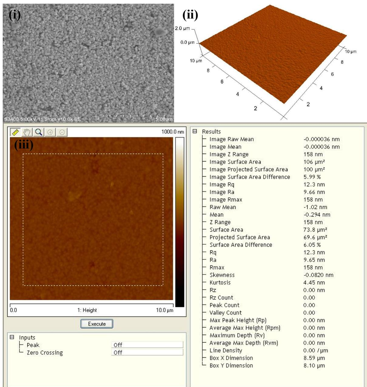
**Fig. S2** (i) SEM image and (ii) AFM image of gold film of  $\sim 100$  nm thickness electrochemically deposited onto silicon wafers coated with  $1000 \text{ \AA}$  gold (Au)  $525 \text{ \mu m}$  thickness over a  $50 \text{ \AA}$  titanium adhesion layer. (Bottom) Surface roughness measurement example suggesting the unmodified gold surface is rough with a root mean square (RMS) roughness of  $12.3 \text{ nm}$  (average RMS roughness was found to be  $12.13 \pm 0.27$ ).
