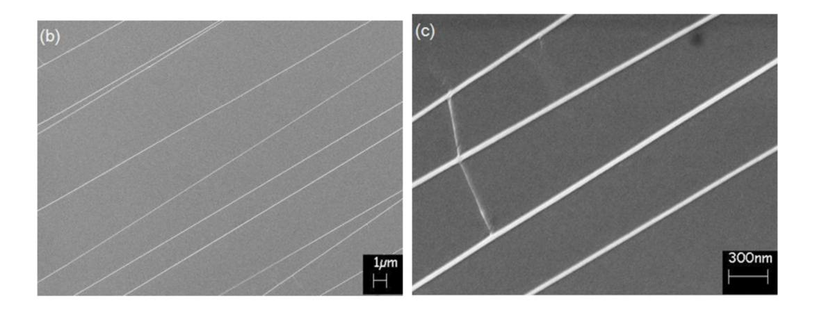
Figure 5.3 (a) Schematic diagram of scanning electrospinning set-up (b) and (c) SEM images of aligned ZrO<sub>2</sub> nanofibers fabricated by scanning electrospinning
