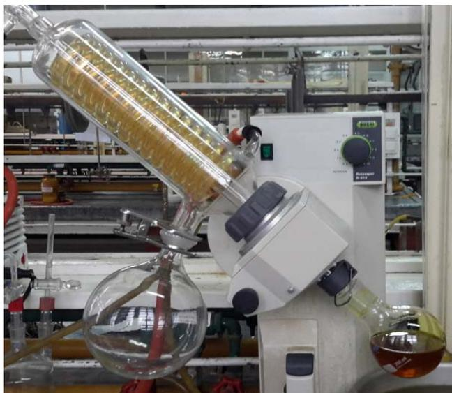
**SM 11.1.2** – Rotary evaporator for methanol removal
