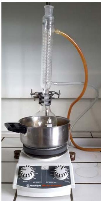
**SM 11.1.1** – Reaction set-up apparatus for 4-bromomethylbenzoic acid
